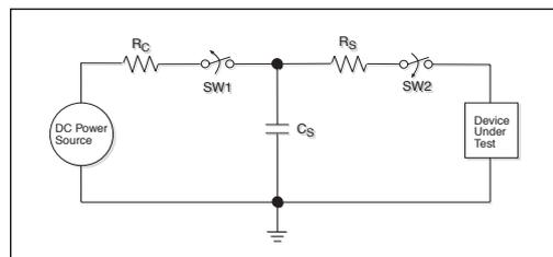
Figure 6. ESD Test Circuit for Human Body Model
