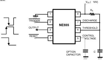
Fig. 2. Monostable Operation
