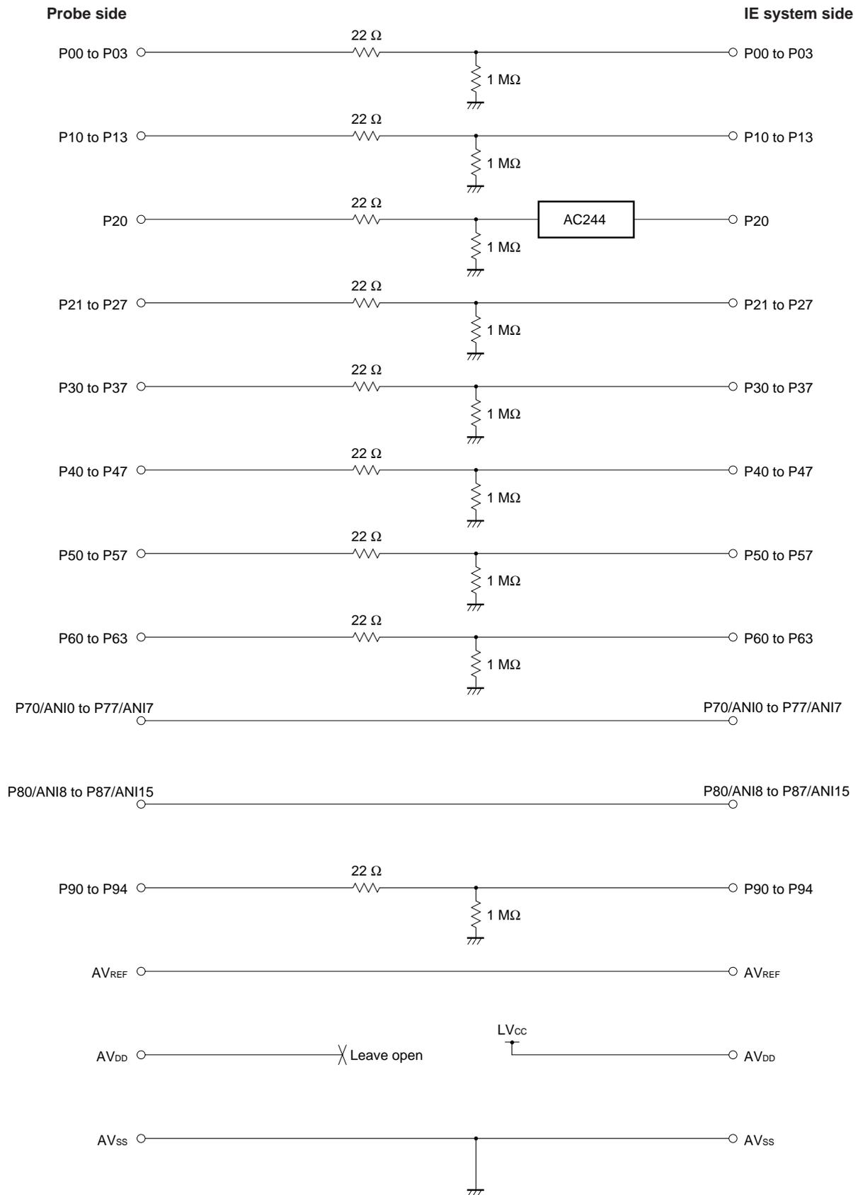
**(2) Signals input from the target system via a gate**
