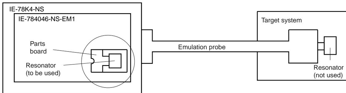
**Remark** The clock that is supplied by the IE-784046-NS-EM1's resonator (encircled in the figure) is used.
