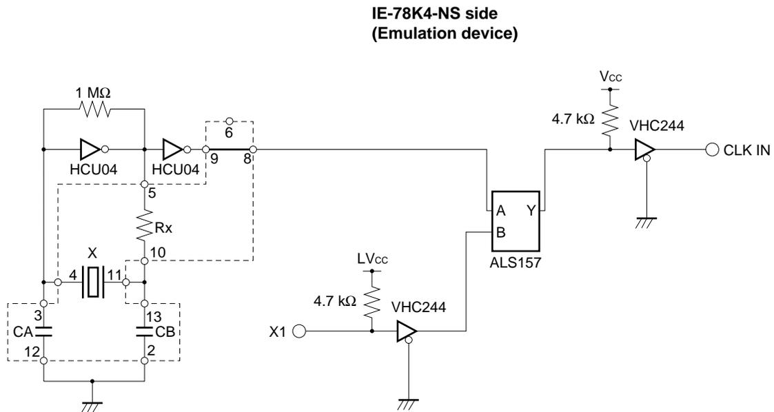
**Remark** The sections enclosed in broken lines indicate parts that are attached to the parts board.
