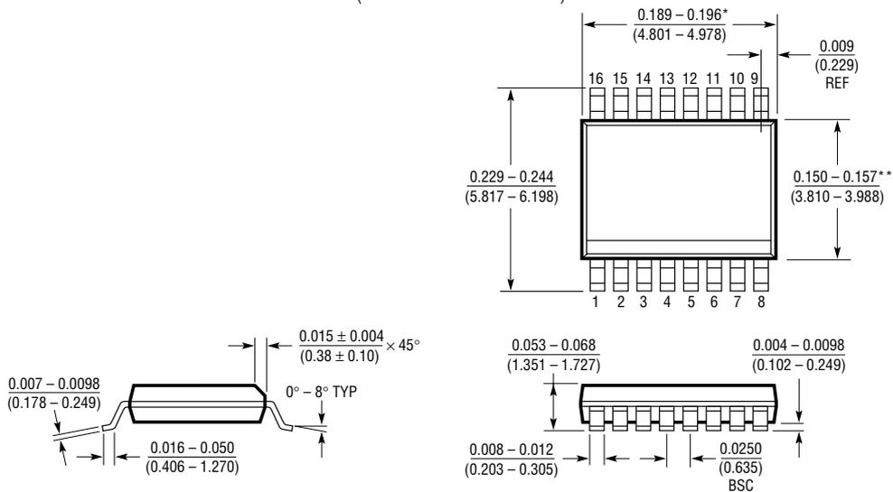
\* DIMENSION DOES NOT INCLUDE MOLD FLASH. MOLD FLASH SHALL NOT EXCEED 0.006" (0.152mm) PER SIDE
