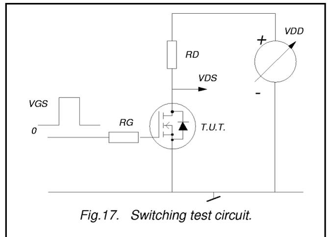
Fig.17. Switching test circuit.
