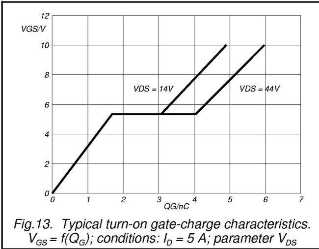
Fig.13. Typical turn-on gate-charge characteristics.
