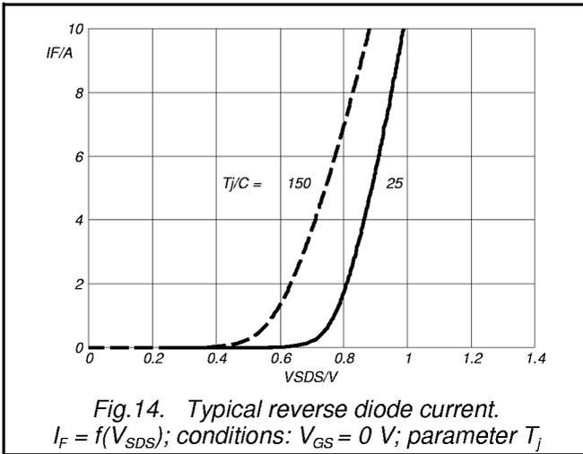
Fig.14. Typical reverse diode current.
