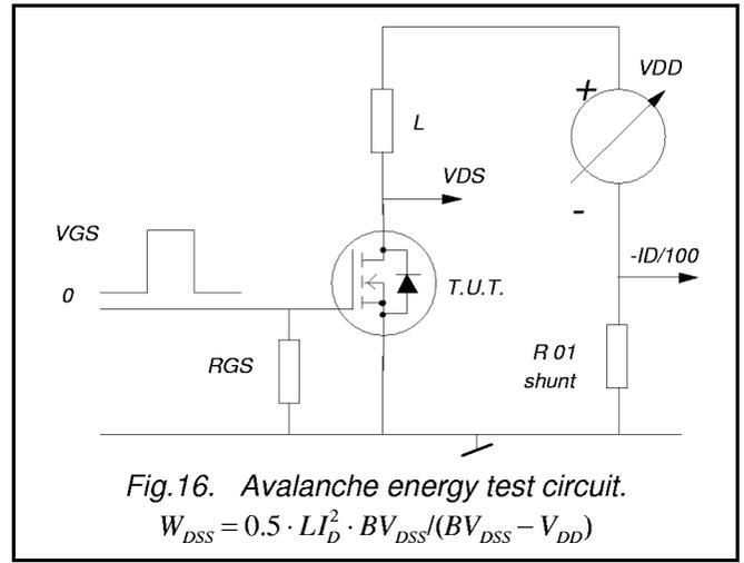
Fig.16. Avalanche energy test circuit.
