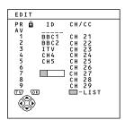
3 Press the V/▲ buttons to choose the first character of a Channel name (ID) you want to attach to the TV channel.
