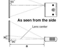
**a** (min length) = projection size (inches)  $\times$  0.04064 **a** (max length) = projection size (inches)  $\times$  0.04878
