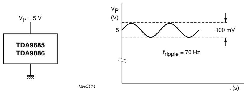
Fig.6 Ripple rejection condition.
