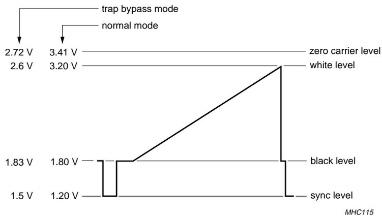
Fig.5 Typical video signal levels on output pin CVBS (sound carrier off).
