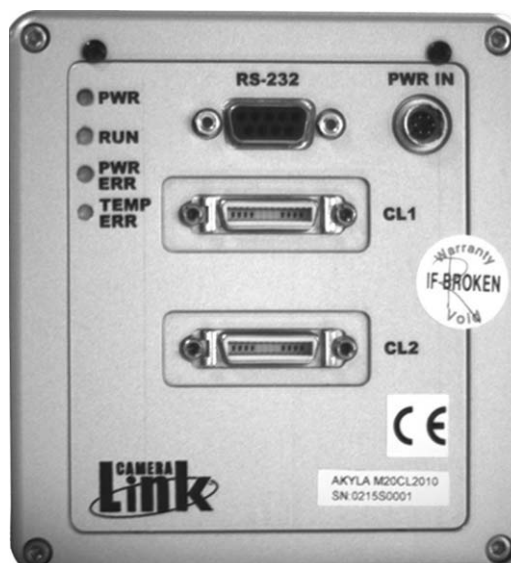
Figure 14. Rear Panel Layout for CameraLink Models
