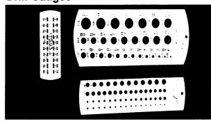
Manufactured from hardened and ground steel. Satin chrome finish for protection and easy reading. English and metric styles available.
