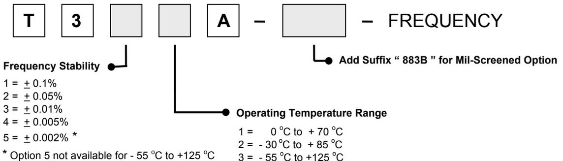
**EXAMPLE: T343A - 883B - 24.000 MHz = 14 Pin Package, 100K ECL, ± 0.005% over -55 °C to +125 °C, Mil-Screened , and 24.000 MHz**
