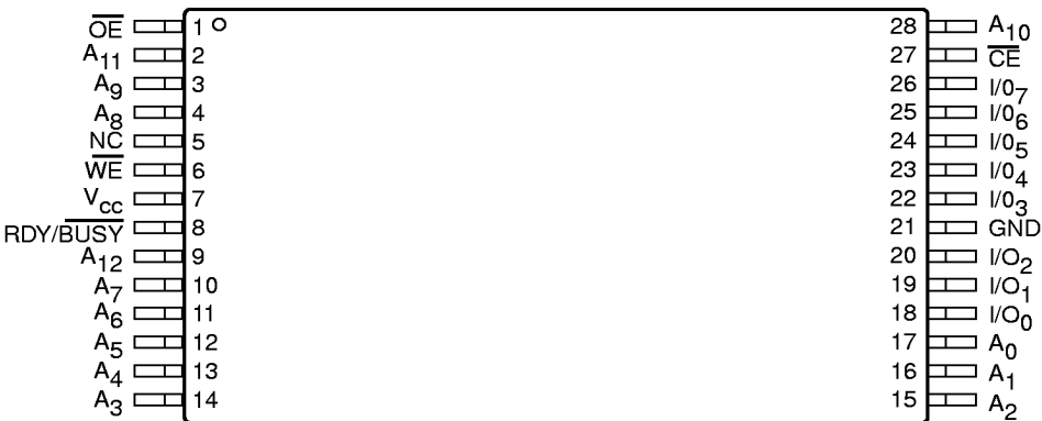
TSOP Top View (8mm x 13.4mm) (T13)
