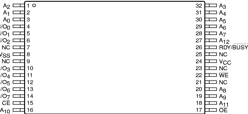
TSOP Top View (8mm x 14mm) (T14) TSOP Top View (8mm x 20mm) (T)
