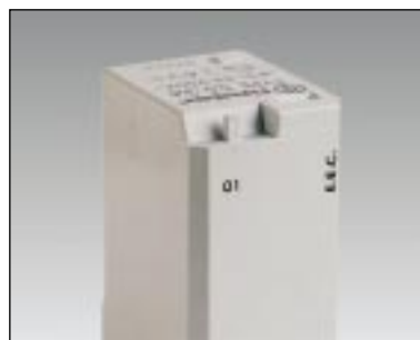
REMOVE VENTILATION PIP The sealed version has a removable pip to avoid ozone accumulation when relay is operating.
