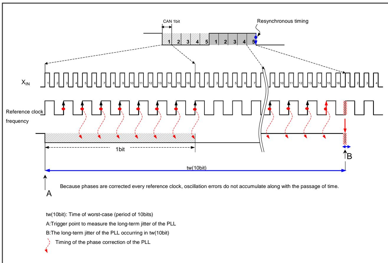
Figure 3 Relation of resynchronization on CAN communication and PLL phase correction
