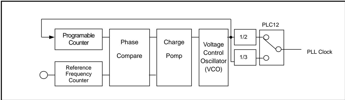
**Figure 1 PLL block diagram**
