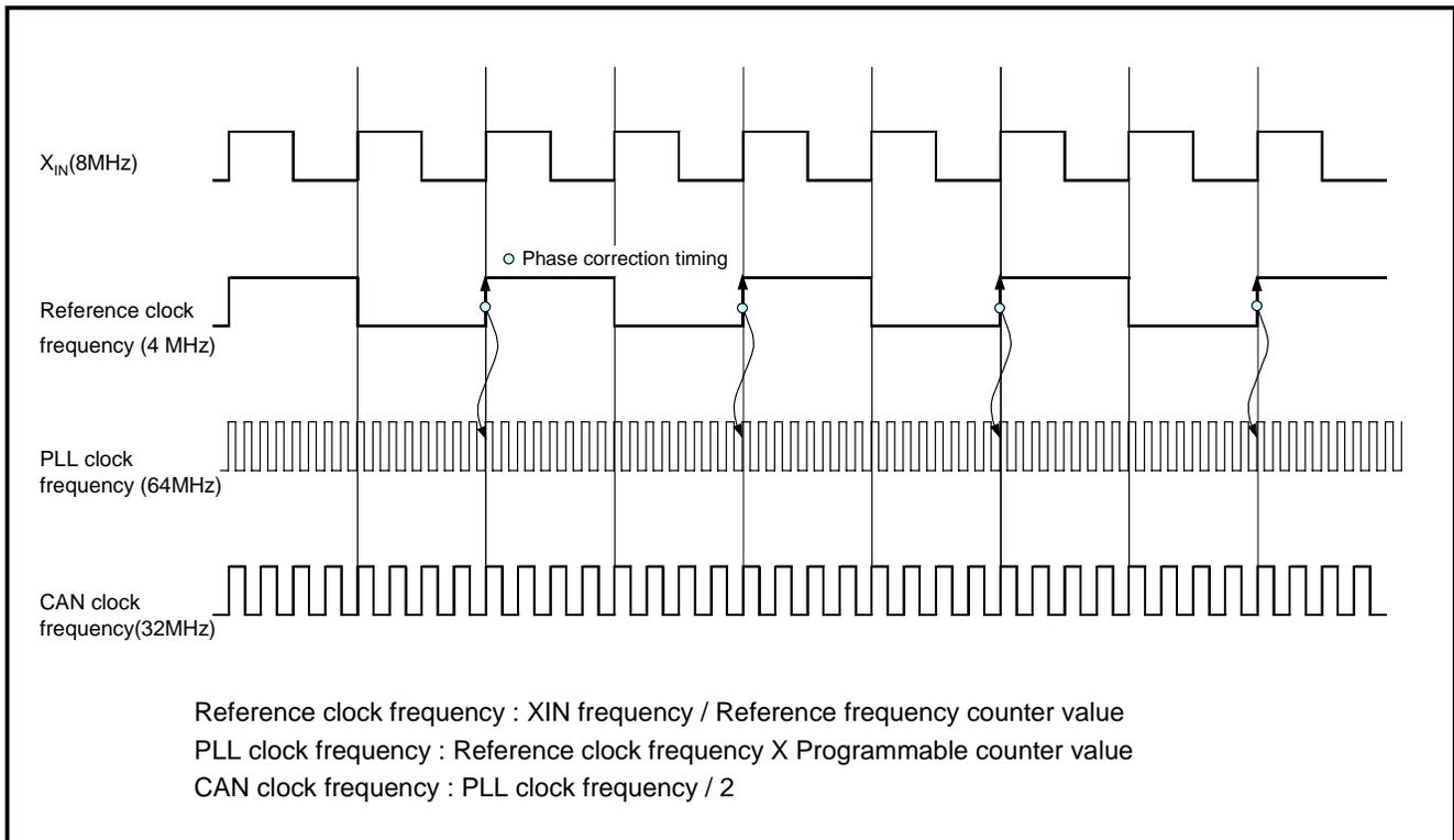
**Figure 2 Phase correction timing**
