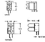
The colour combinations for these types are specified by replacing 'U' and 'L' with the letters R, G, Y or A (red, green, yellow or amber) to denote the Upper and Lower LED colours.
