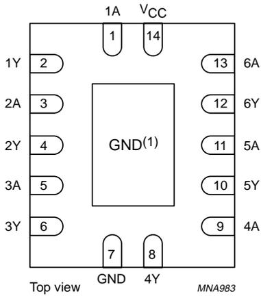
(1) The die substrate is attached to this pad using conductive die attach material. It can not be used as a supply pin or input.
