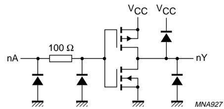
Fig.5 Schematic diagram (one inverter).
