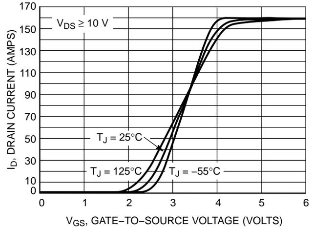
Figure 2. Transfer Characteristics
