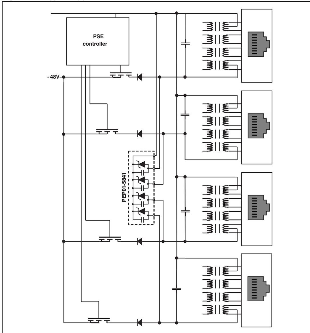
Figure 10 and 11 shows typical application schematics of PoE network. Power sourcing equipment (PSE) allows communication and power sourcing for several power devices (PD). The number of ways is generally a multiple of 4, this optimizes the PEP01-5841 for track layout and crosstalk, as well as PCB surface occupation. This protection device has been studied to comply with the latest IEEE 802.3af-2003 requirements and to withstand the surge defined in the IEC 61000-4-5 level 4 requirements.
