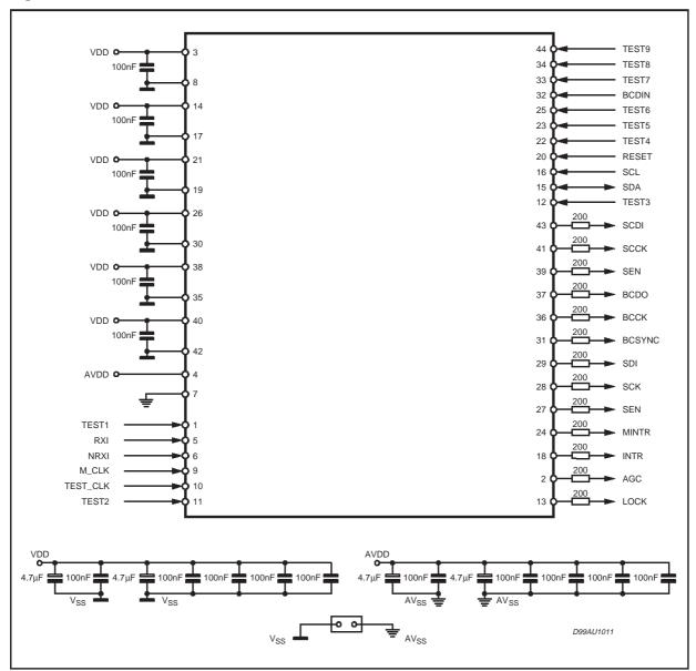
Figure 4. Test Load Circuit
