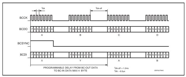
Fig. 8: Format Of The Service Component Interface
