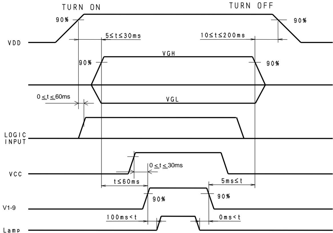
Turn on :VDD → VGL → VGH → Logic input → VCC → V1-V9
