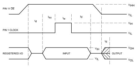
NOTE:  $t_d = t_{SU} = t_W = 100$ ns to 1000ns. VIHH = 10.25V to 10.75V.
