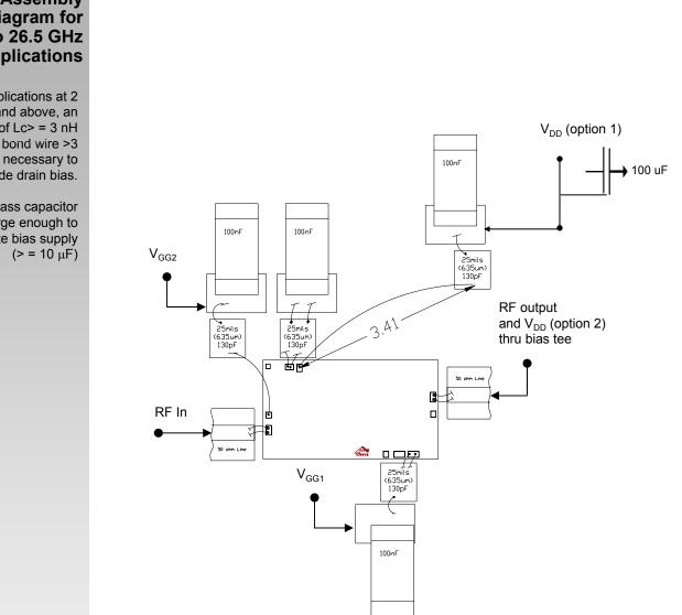
Recommended Assembly **Diagram for** 2 to 26.5 GHz **Applications**
