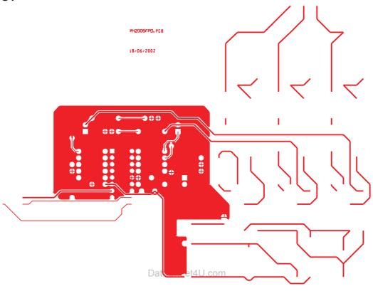
Figure 6: PM2005F Top PCB layout
