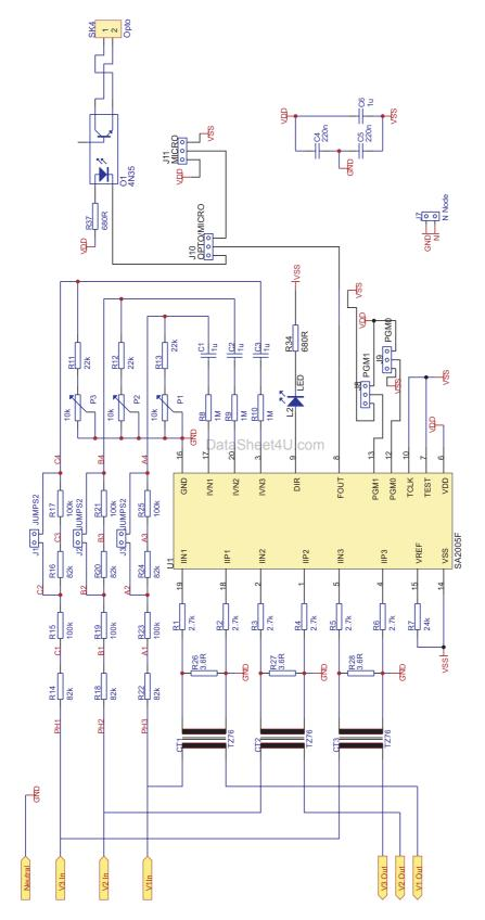
Figure 9: Schematic Diagram for Metering Section
