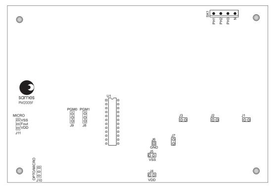
Figure 2: Jumper positions
