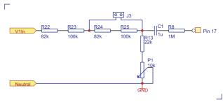
Figure 5: Mains Voltage Divider
