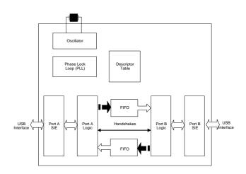
As shown in the block diagram above, this ASIC contains two USB units working independently. Together with the two FIFOs and control logic in between, they exchange data without blocking. The entire clock oscillator, PLL, voltage regulators, USB transceivers, and power-on reset circuits are integrated on the chip. There is no glue logic needed.
