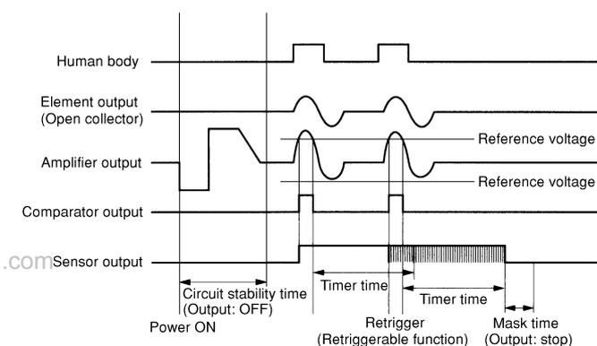
\* "Mask time" is included to prevent malfunctions caused by fluctuations in the load current at the moment the timer stops operation. During the "Mask time", the output from the sensor is turned off.
