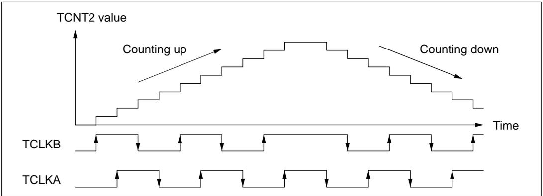
**Figure 8-44 Operation in Phase Counting Mode (Example)**
