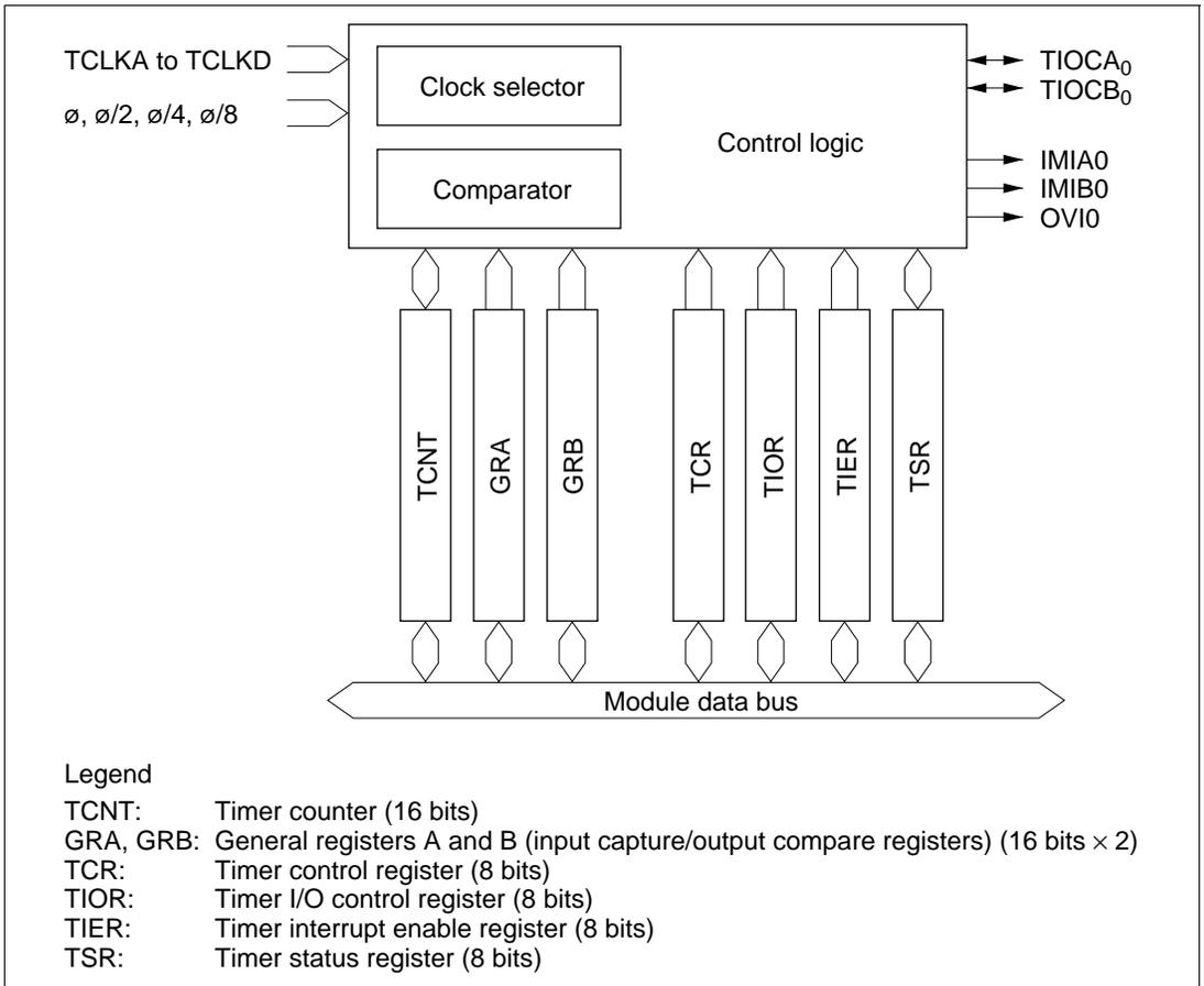
**Figure 8-2 Block Diagram of Channels 0 and 1 (for Channel 0)**
