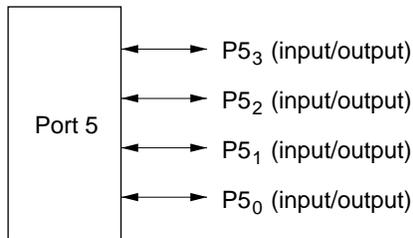
**Figure 7-15 Pin Functions in Mode 6 and 7 (Port 5)**
