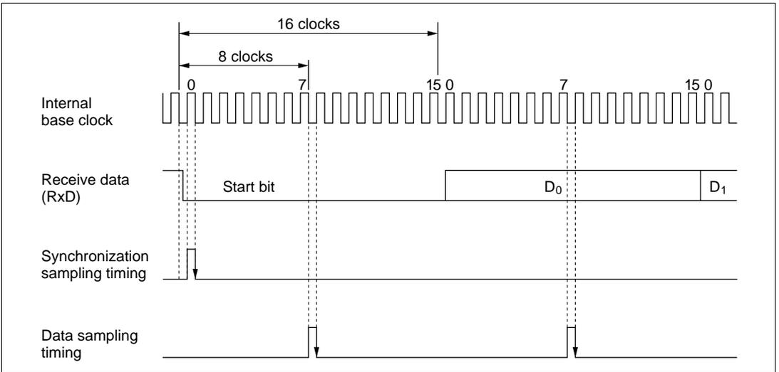
**Figure 11-21 Receive Data Sampling Timing in Asynchronous Mode**
