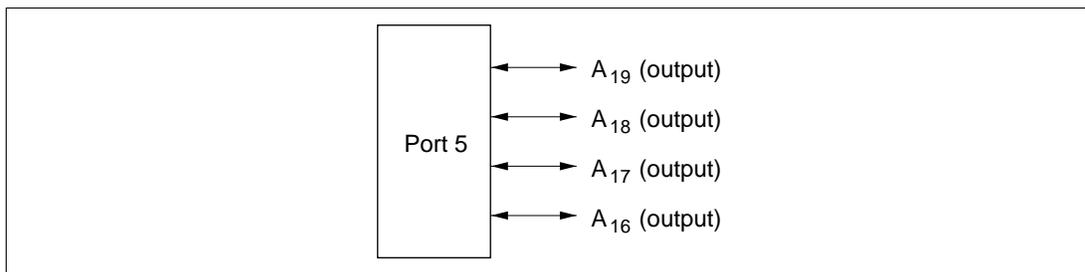
**Figure 7-13 Pin Functions in Modes 1 and 3 (Port 5)**
