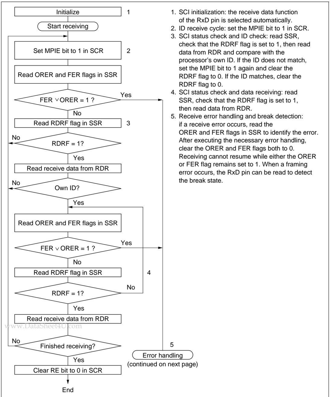
**Figure 11-12 Sample Flowchart for Receiving Multiprocessor Serial Data (1)**
