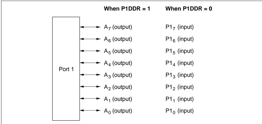
**Figure 7-3 Pin Functions in Mode 5 (Port 1)**
