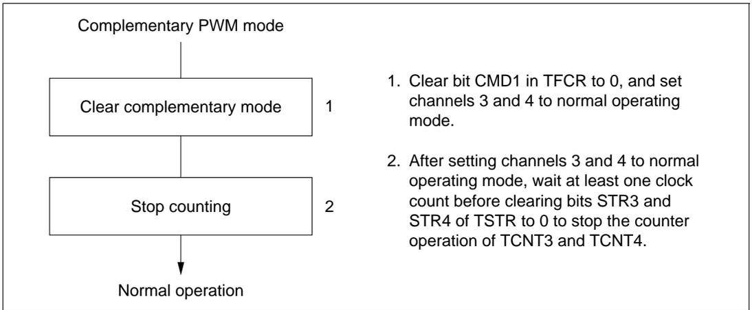
**Figure 8-34 Clearing Procedure for Complementary PWM Mode (Example)**
