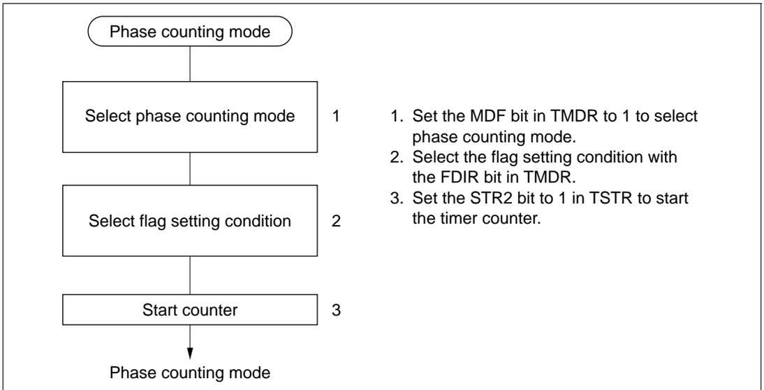
**Figure 8-43 Setup Procedure for Phase Counting Mode (Example)**
