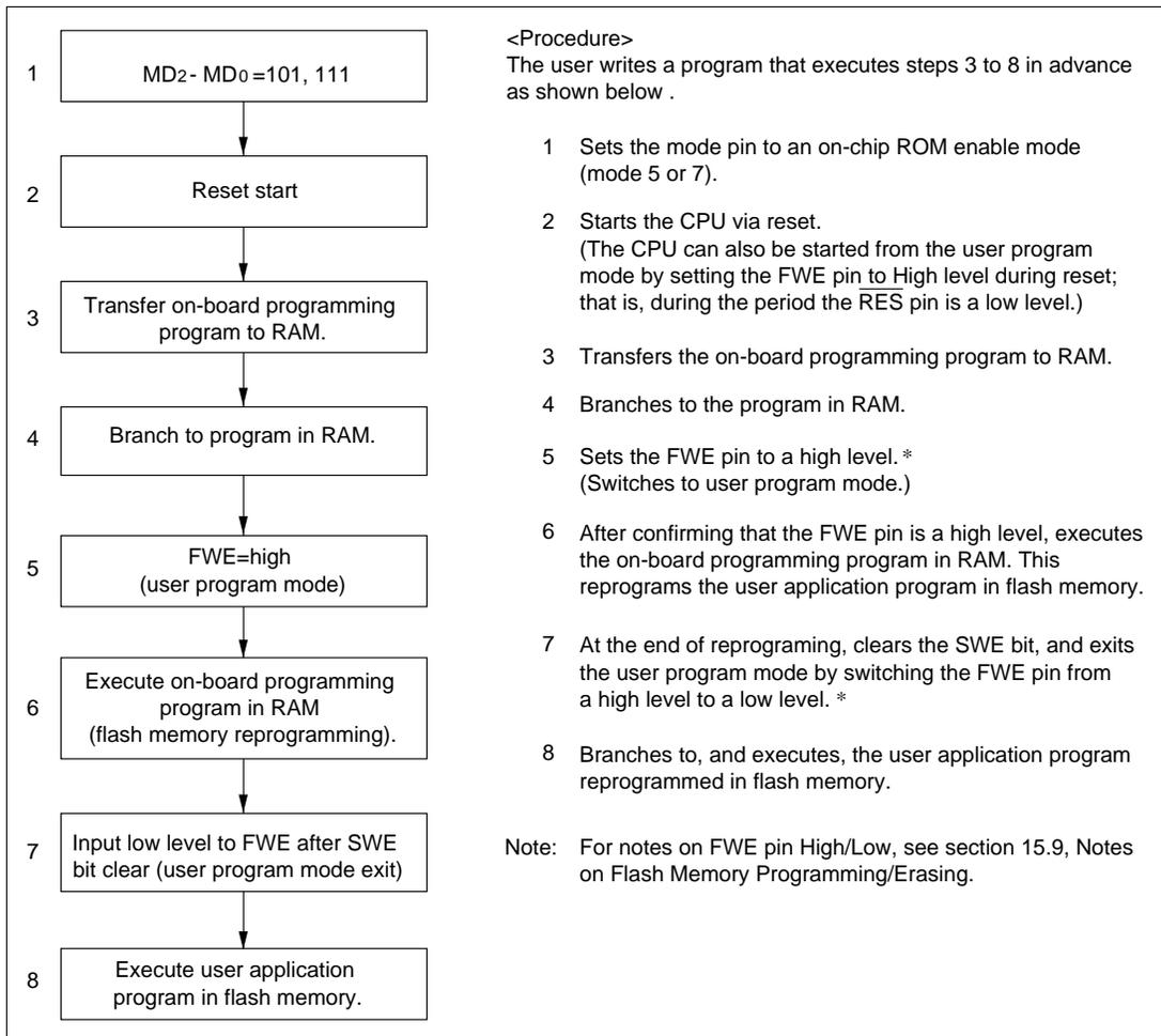
**Figure 15-9 User Program Mode Execution Procedure (Example)**
