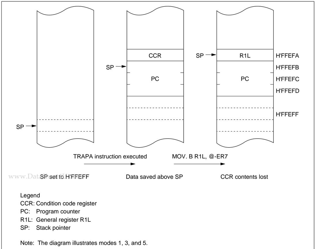
Figure 4-5 Operation when SP Value is Odd [www.DataSheet4U.com](http://www.DataSheet4U.com)
