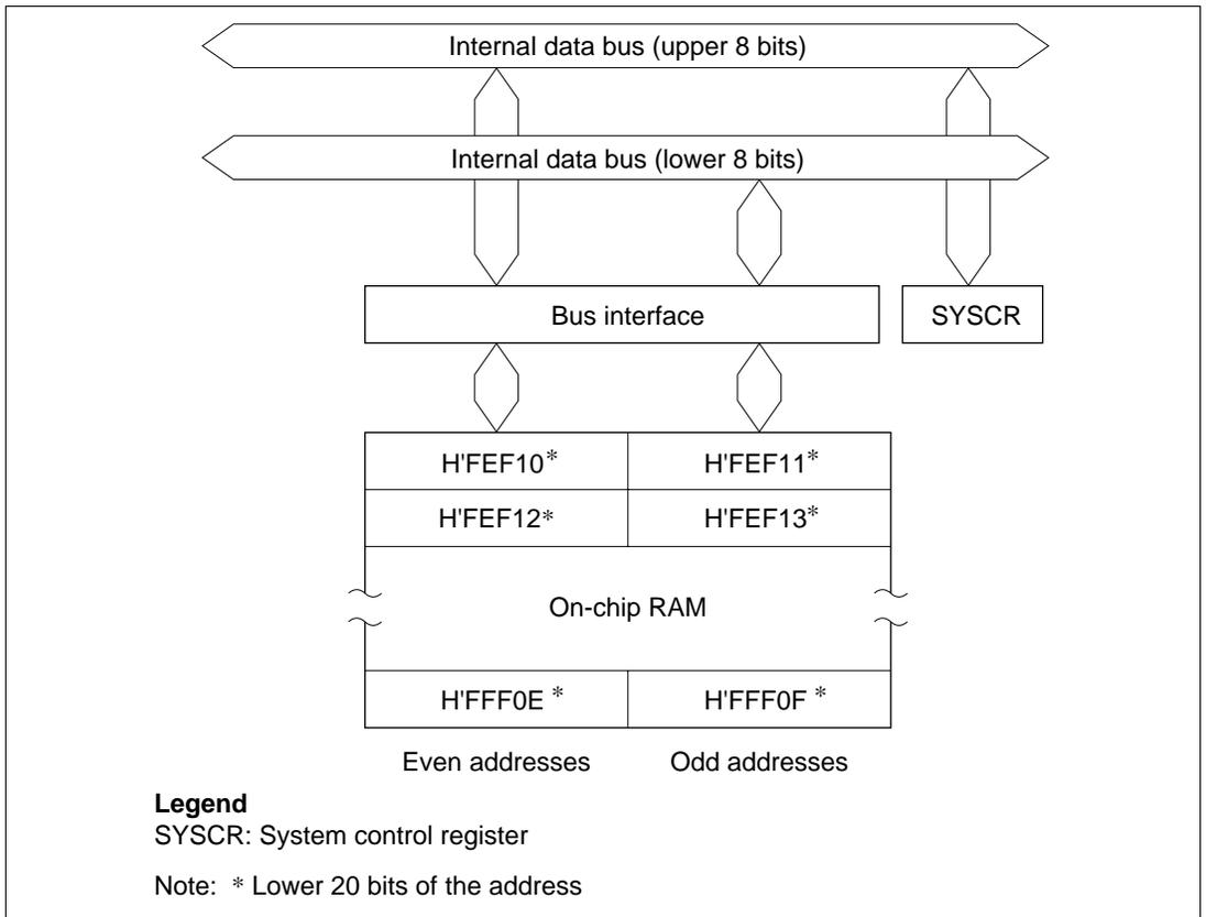
**Figure 14-1 RAM Block Diagram (H8/3039 in Modes 1, 5 and 7)**
