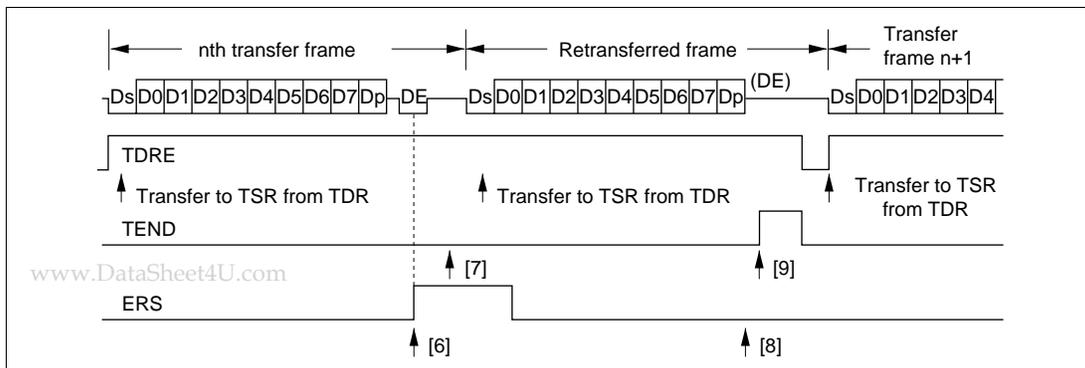
**Figure 12-9 Retransfer Operation in SCI Transmit Mode**
