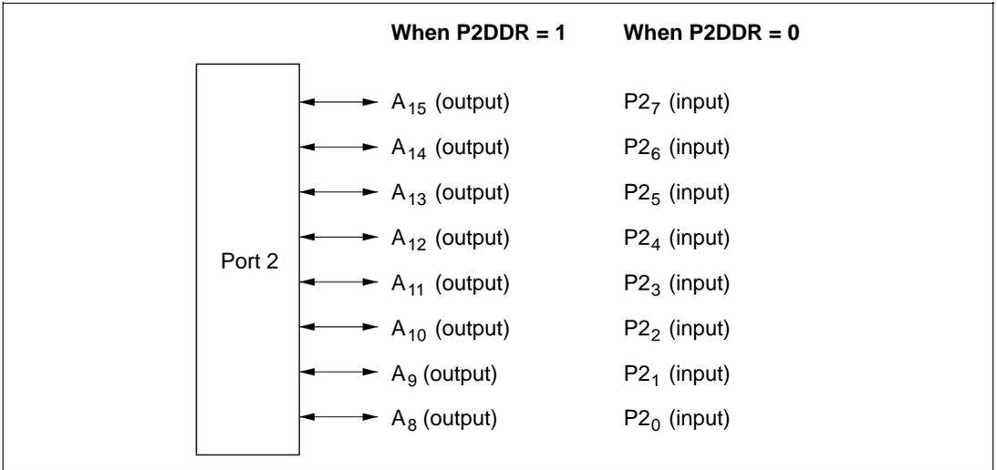
**Figure 7-7 Pin Functions in Modes 1 and 3 (Port 2)**
