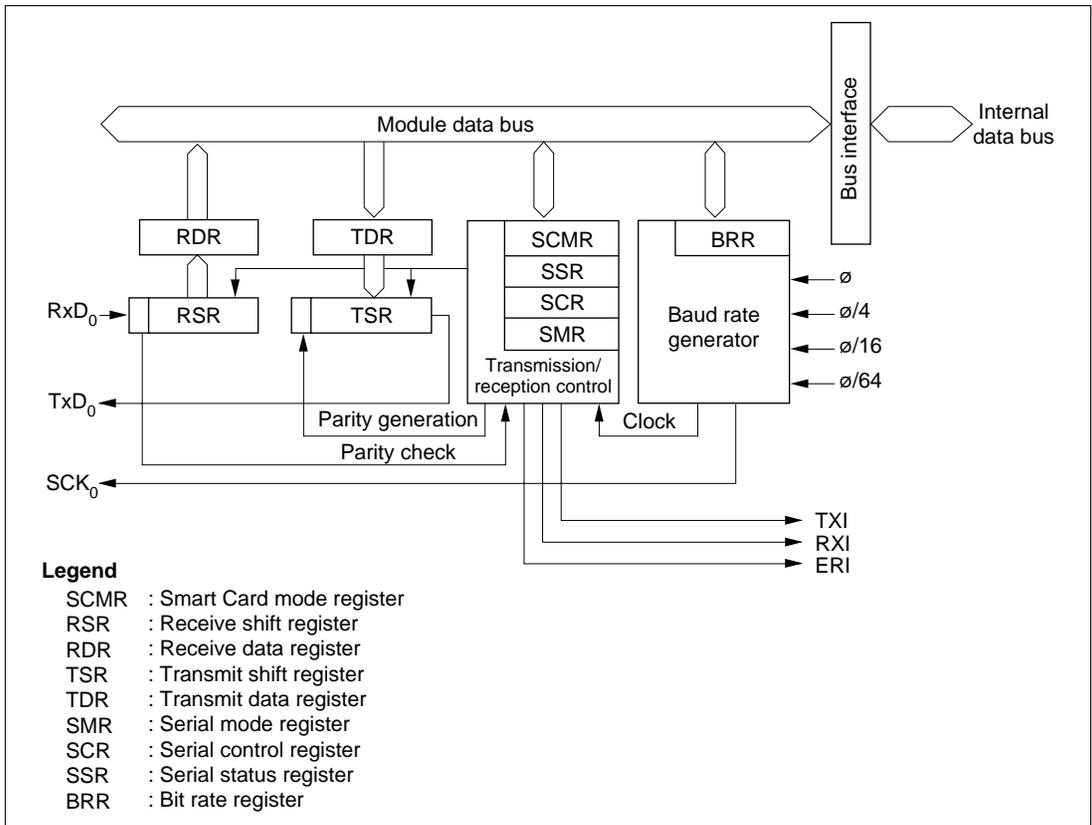
**Figure 12-1 Block Diagram of Smart Card Interface**
