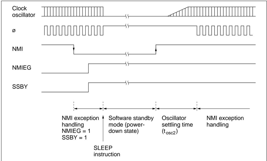
Figure 17-1 NMI Timing for Software Standby Mode (Example)
