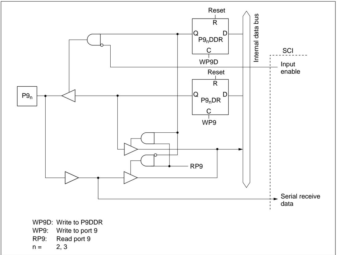
**Figure C-8 (c) Port 9 Block Diagram (Pin P9<sub>2</sub>, P9<sub>3</sub>)**
