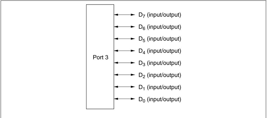
**Figure 7-10 Pin Functions in Modes 1, 3 and 5 (Port 3)**
