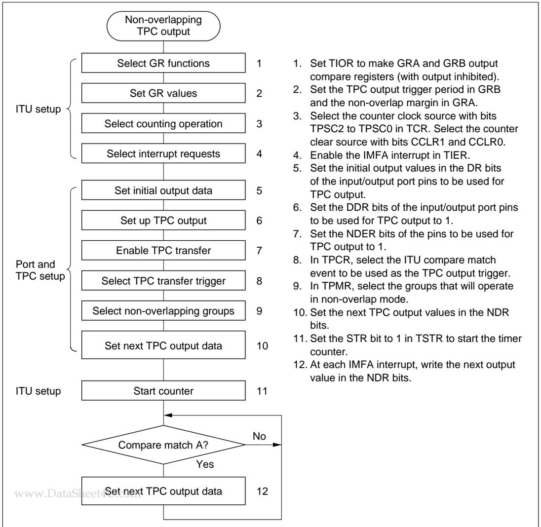
**Figure 9-6 Setup Procedure for Non-Overlapping TPC Output (Example)**
