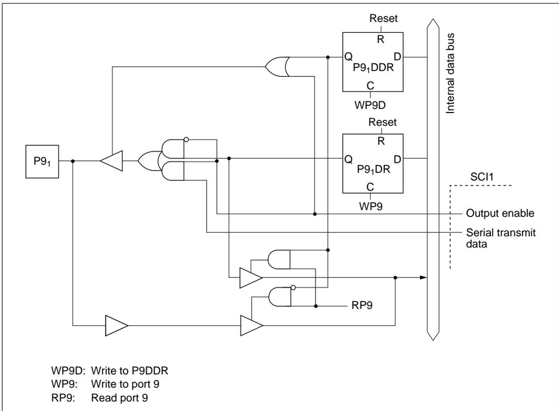
**Figure C-8 (b) Port 9 Block Diagram (Pin P9<sub>1</sub>)**
