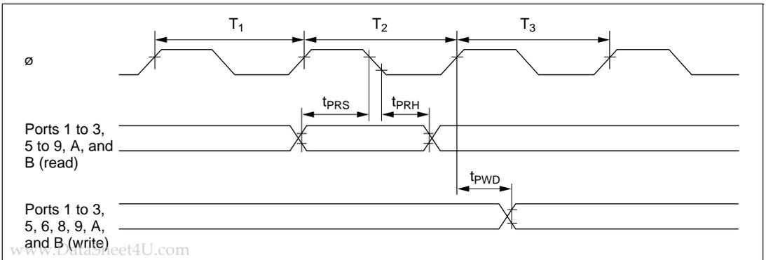
Figure 18-14 TPC and I/O Port Input/Output Timing
