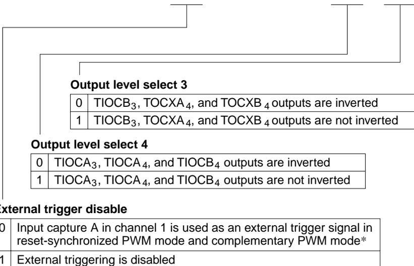
Note: \* When an external trigger occurs, bits 5 to 0 in TOER are cleared to 0, disabling ITU output.
