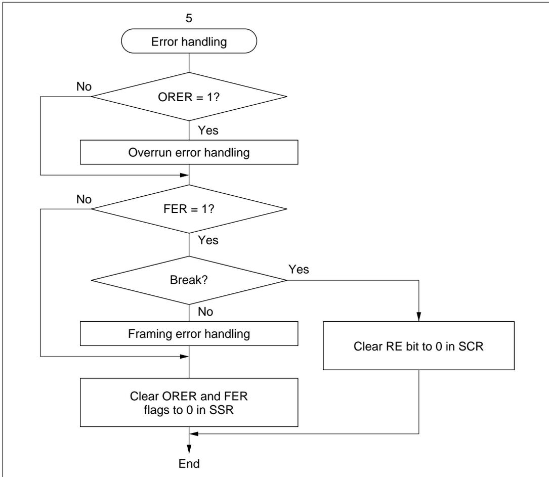
**Figure 11-12 Sample Flowchart for Receiving Multiprocessor Serial Data (2)**
