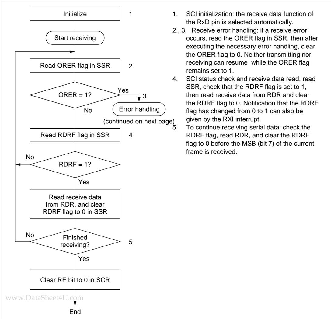
**Figure 11-18 Sample Flowchart for Serial Receiving (1)**
