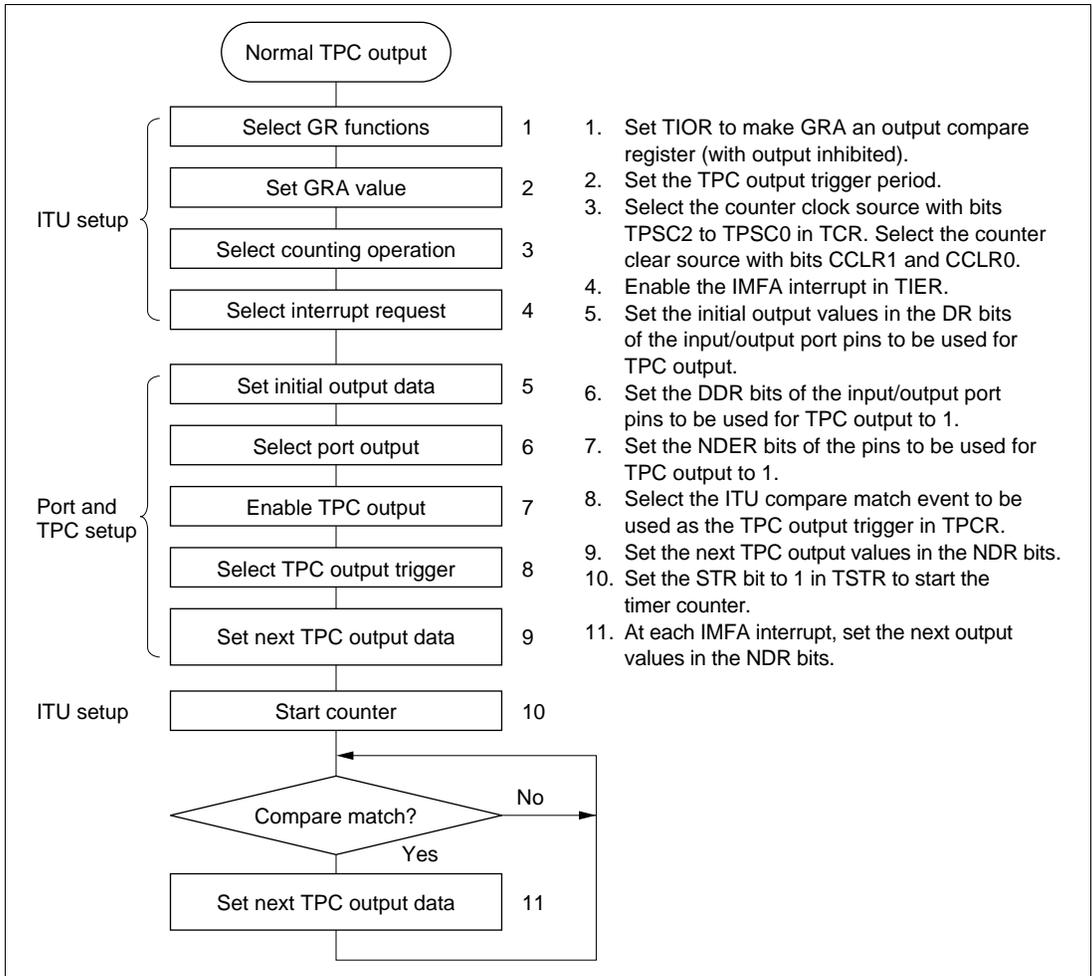
**Figure 9-4 Setup Procedure for Normal TPC Output (Example)**
