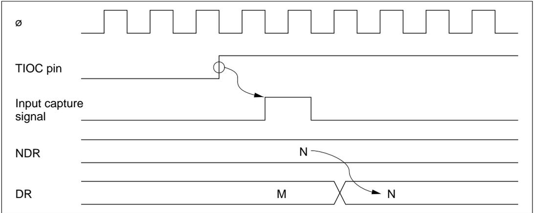
**Figure 9-8 TPC Output Triggering by Input Capture (Example)**
