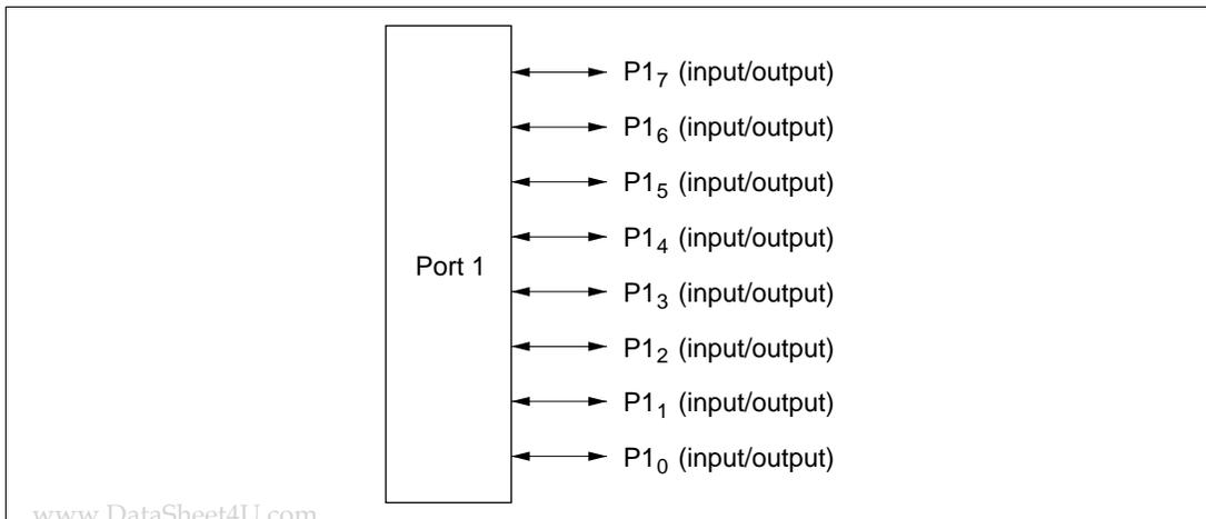
**Figure 7-4 Pin Functions in Modes 6 and 7 (Port 1)**
