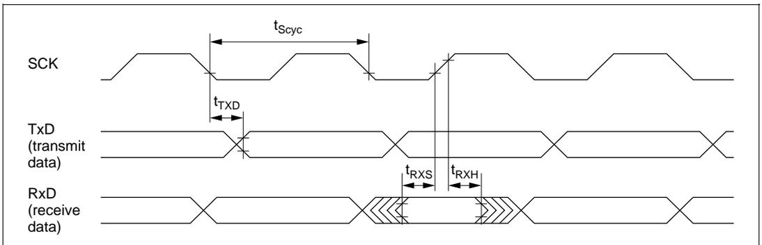
**Figure 18-18 SCI Input/Output Timing in Synchronous Mode**
