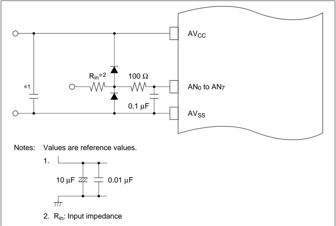
**Figure 13-7 Example of Analog Input Protection Circuit**
