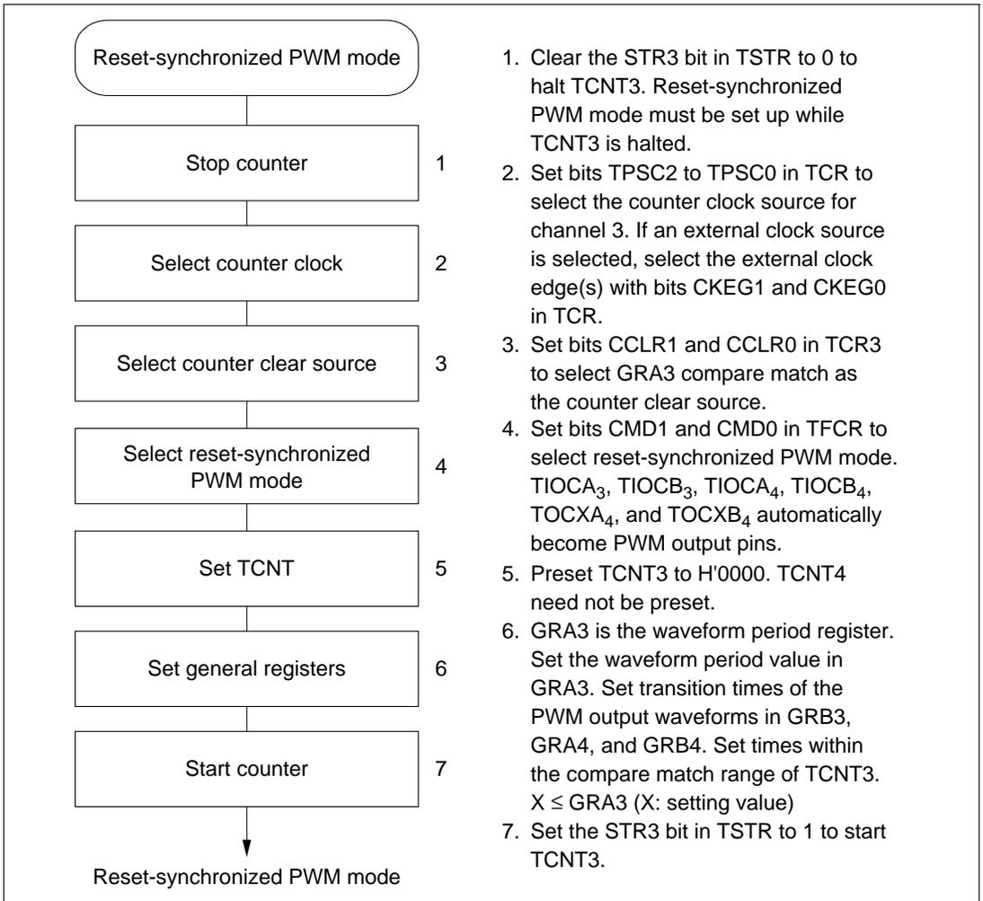
**Figure 8-31 Setup Procedure for Reset-Synchronized PWM Mode (Example)**
