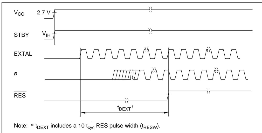
**Figure 16-7 External Clock Output Stabilization Delay Time**
