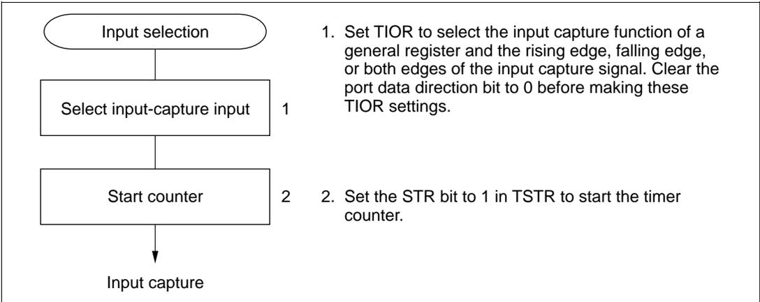
**Figure 8-23 Setup Procedure for Input Capture (Example)**
