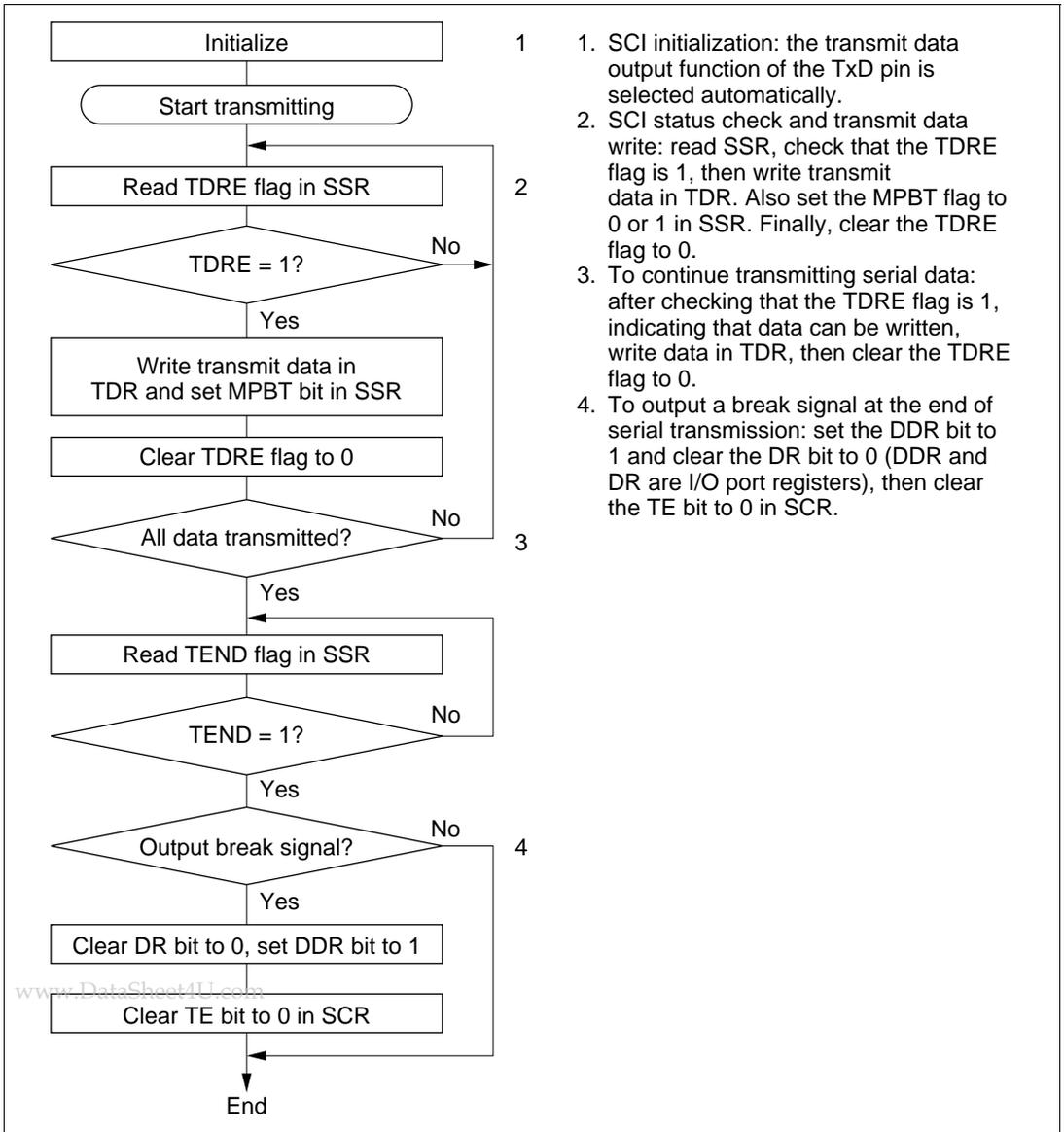
**Figure 11-10 Sample Flowchart for Transmitting Multiprocessor Serial Data**
