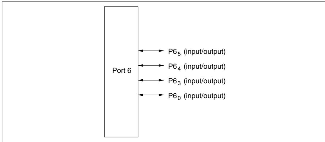
**Figure 7-18 Pin Functions in Modes 6 and 7 (Port 6)**
