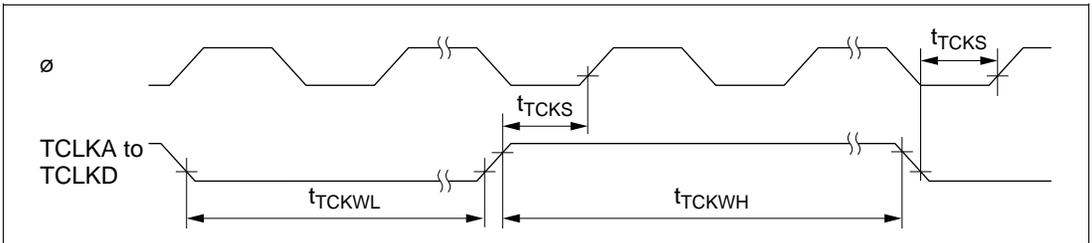
**Figure 18-16 ITU External Clock Input Timing**
