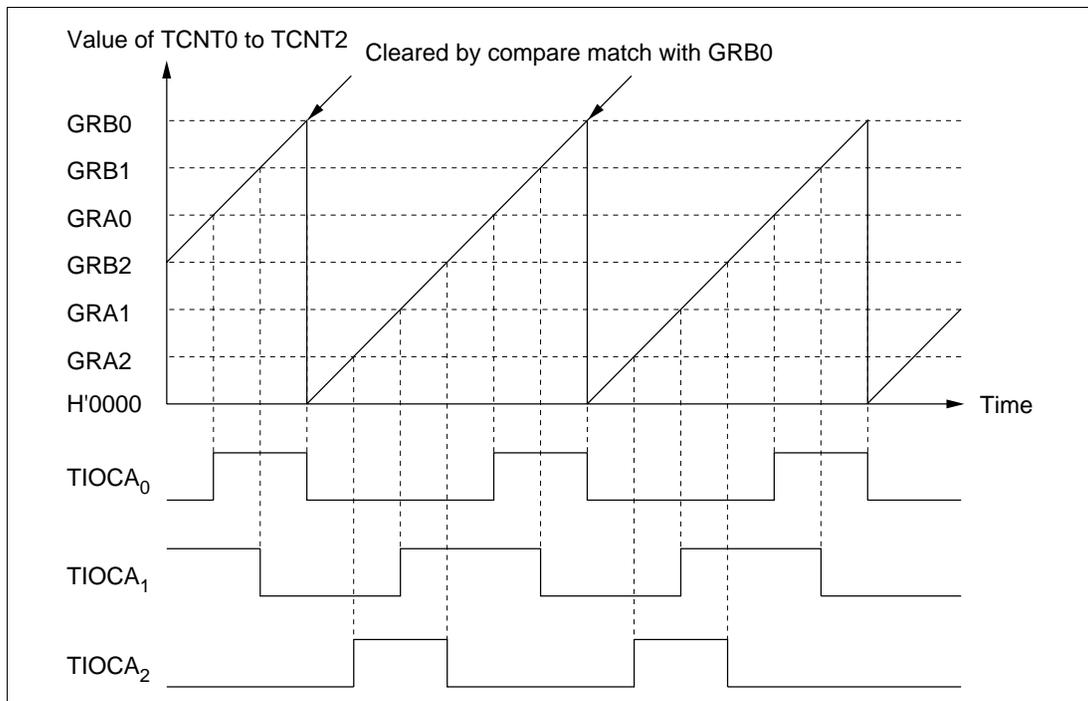
**Figure 8-27 Synchronization (Example)**
