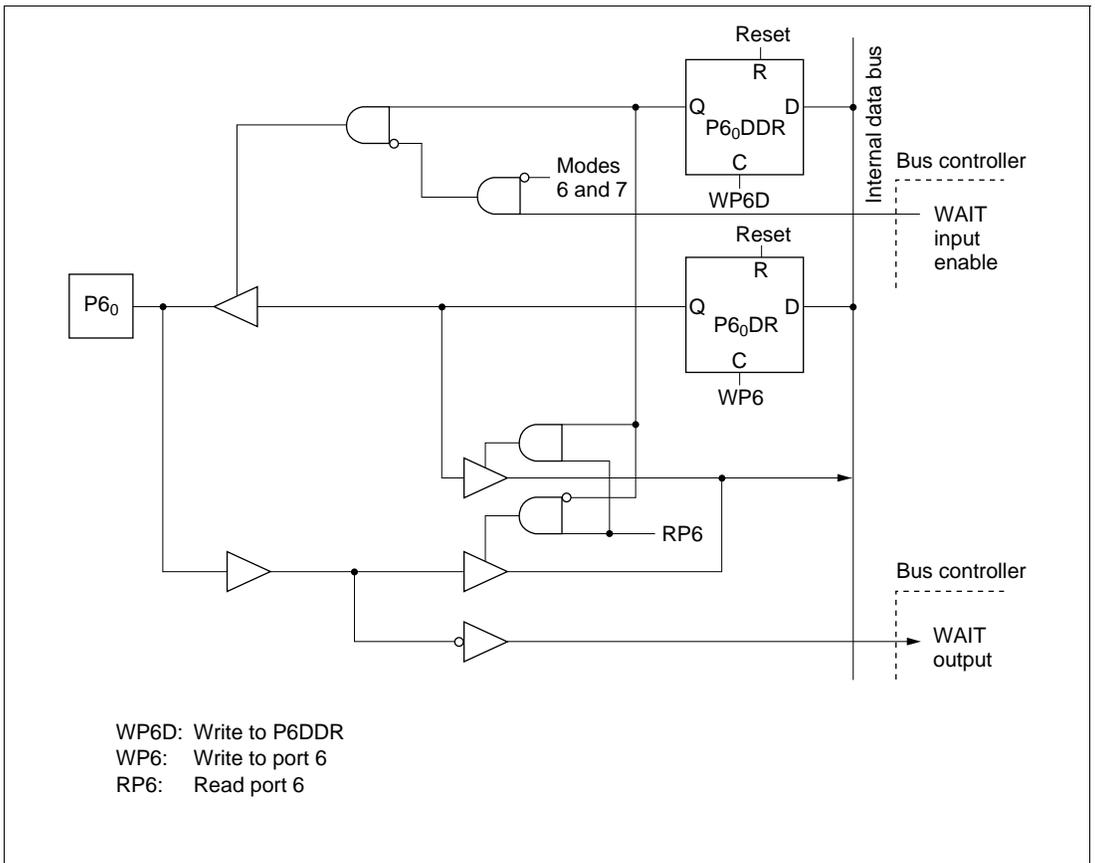
**Figure C-5 (a) Port 6 Block Diagram (Pin P6<sub>0</sub>)**
