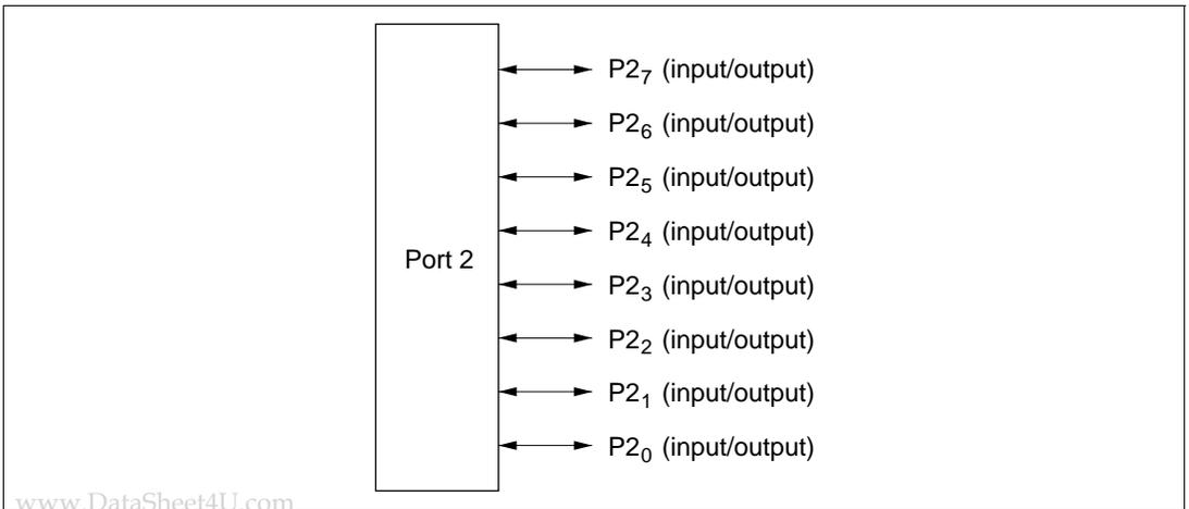
**Figure 7-8 Pin Functions in Modes 6 and 7 (Port 2)**
