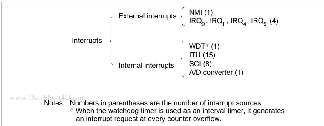
**Figure 4-3 Interrupt Sources and Number of Interrupts**
