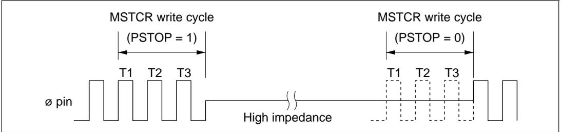
**Figure 17-3 Starting and Stopping of System Clock Output**
