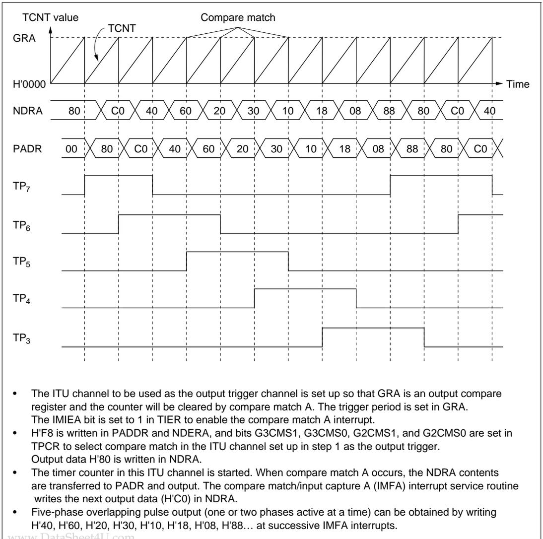
**Figure 9-5 Normal TPC Output Example (Five-Phase Pulse Output)**
