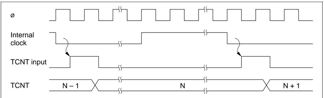
**Figure 8-17 Count Timing for Internal Clock Sources**
