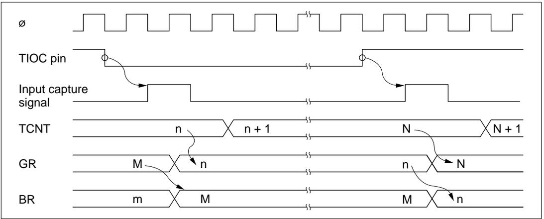
**Figure 8-52 Input Capture and Buffer Transfer Timing (Example)**
