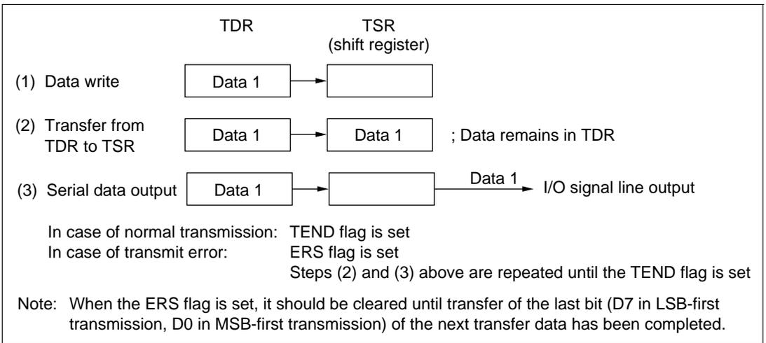
**Figure 12-5 Relation Between Transmit Operation and Internal Registers**
