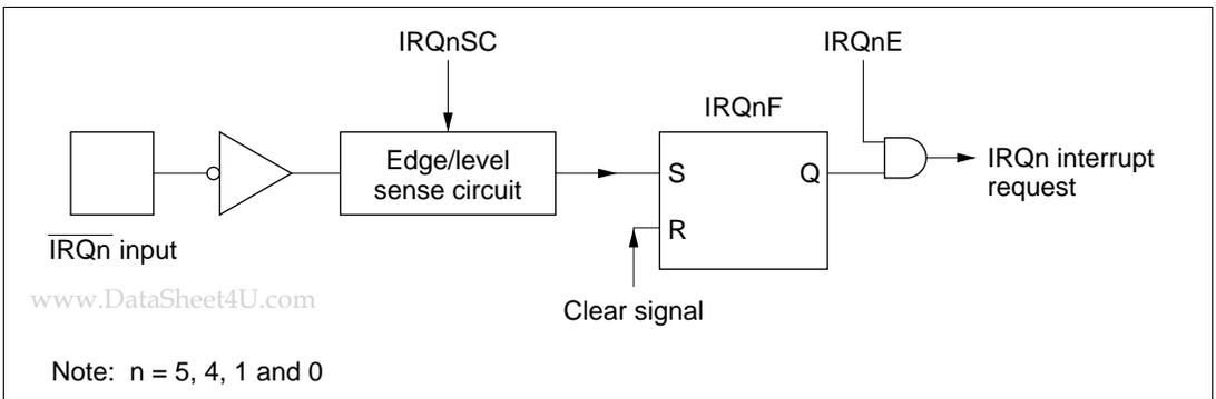
**Figure 5-2 Block Diagram of Interrupts IRQ<sub>5</sub>, IRQ<sub>4</sub>, IRQ<sub>1</sub>, and IRQ<sub>0</sub>**
