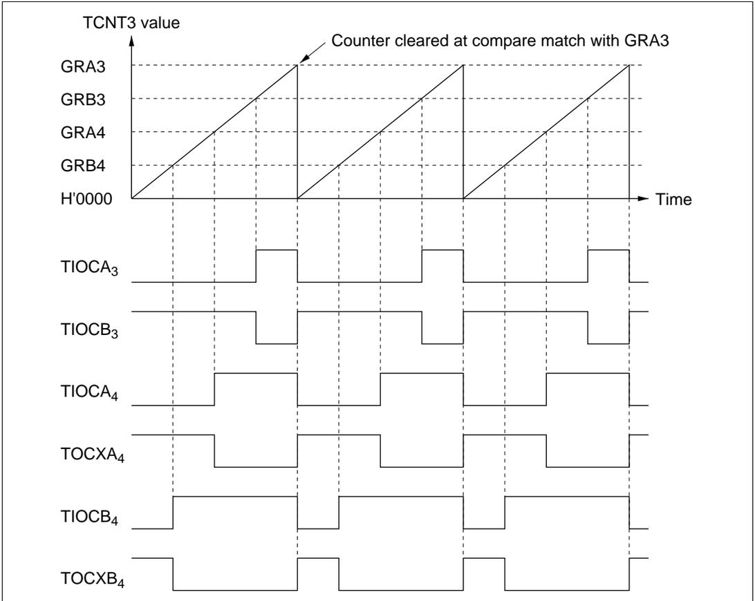
**Figure 8-32 Operation in Reset-Synchronized PWM Mode (Example)**
