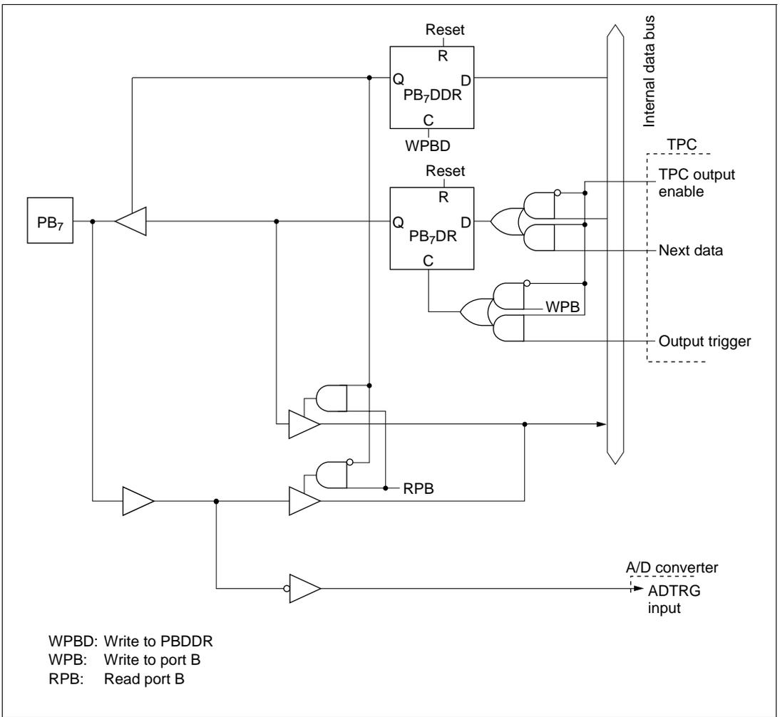
**Figure C-10 (c) Port B Block Diagram (Pin PB<sub>7</sub>)**
