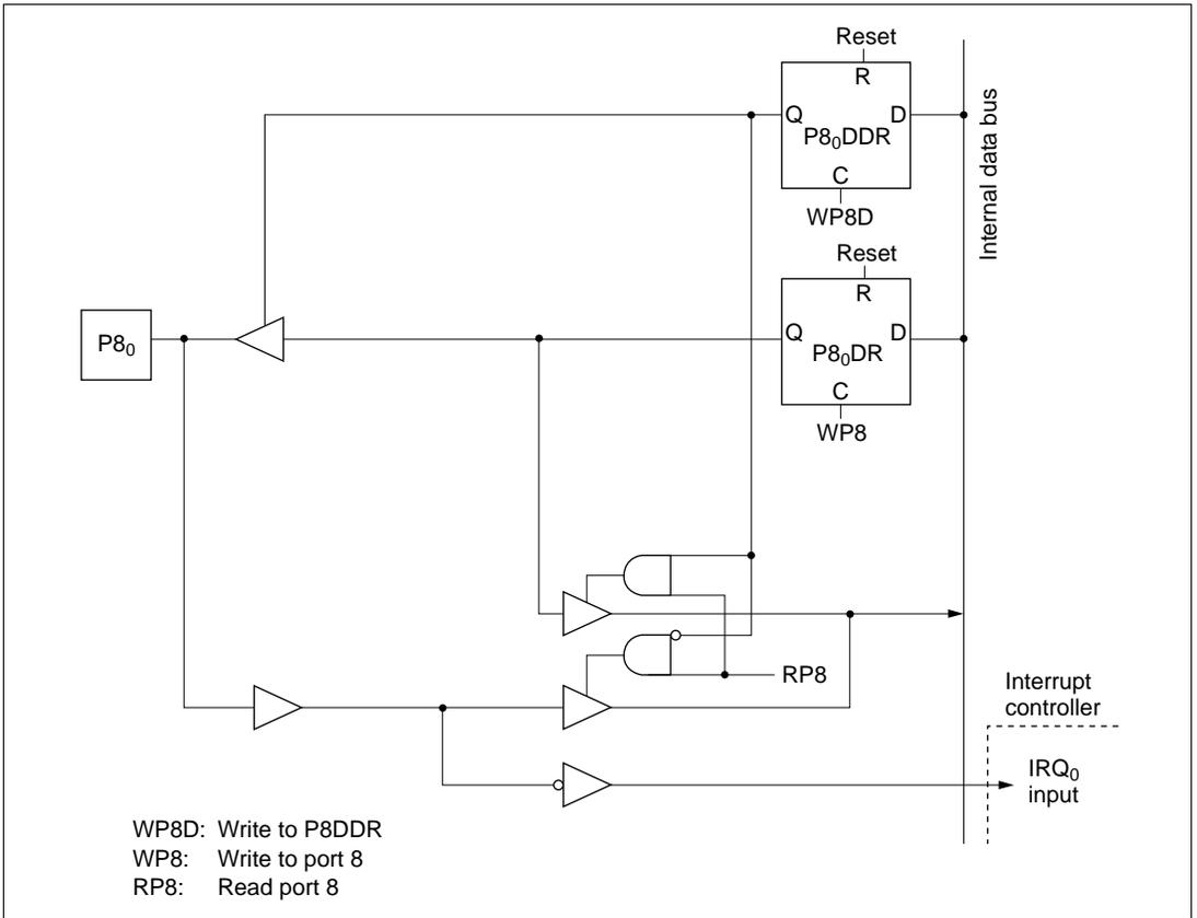
Figure C-7(a) Port 8 Block Diagram (Pin P8<sub>0</sub>)
