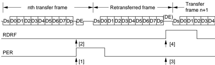
**Figure 12-8 Retransfer Operation in SCI Receive Mode**
