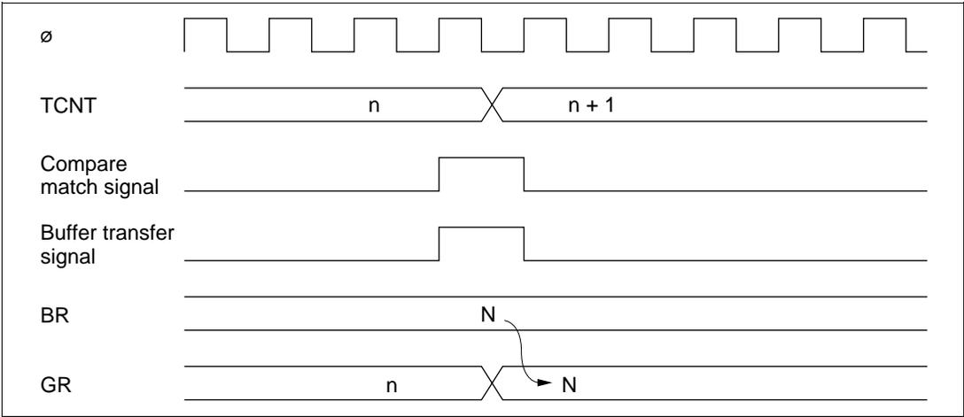
**Figure 8-50 Compare Match and Buffer Transfer Timing (Example)**
