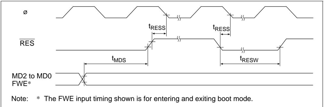
**Figure 18-10 Reset Input Timing**
