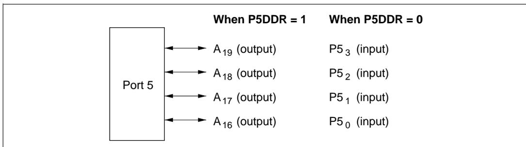
**Figure 7-14 Pin Functions in Mode 5 (Port 5)**
