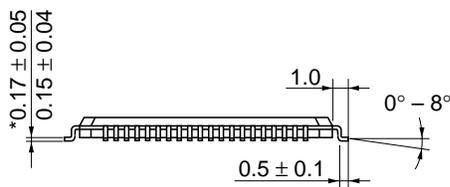
\*Dimension including the plating thickness
