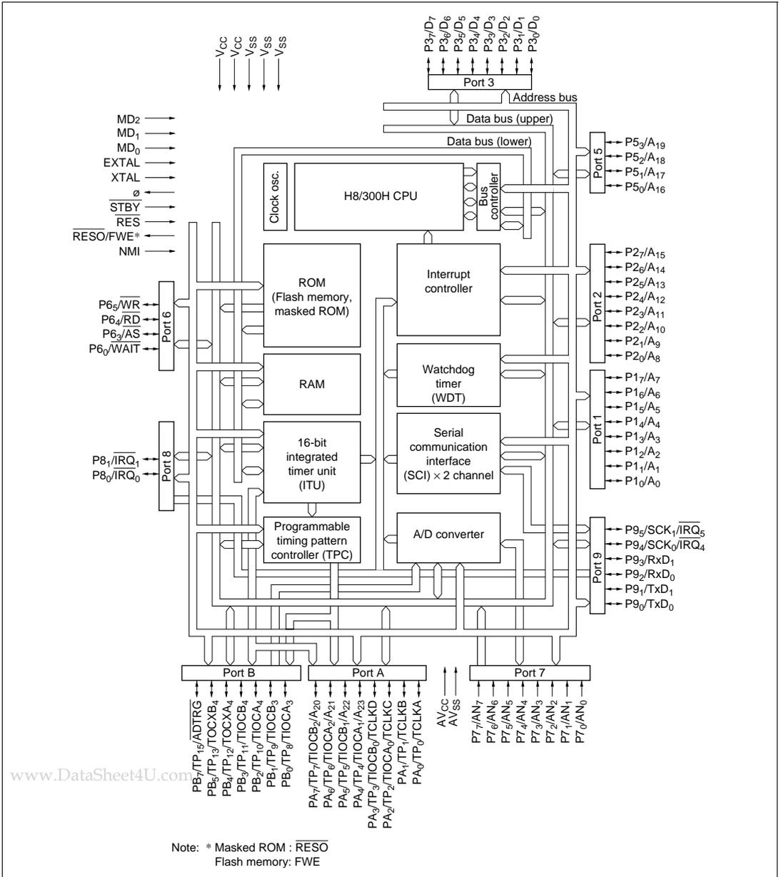
Figure 1-1 Block Diagram
