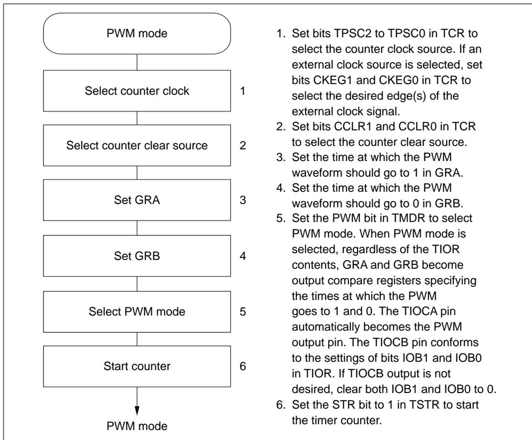
**Figure 8-28 Setup Procedure for PWM Mode (Example)**
