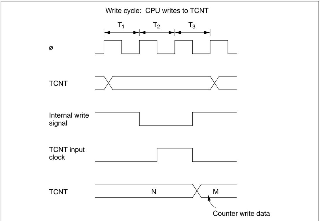
**Figure 10-8 Contention between TCNT Write and Increment**
