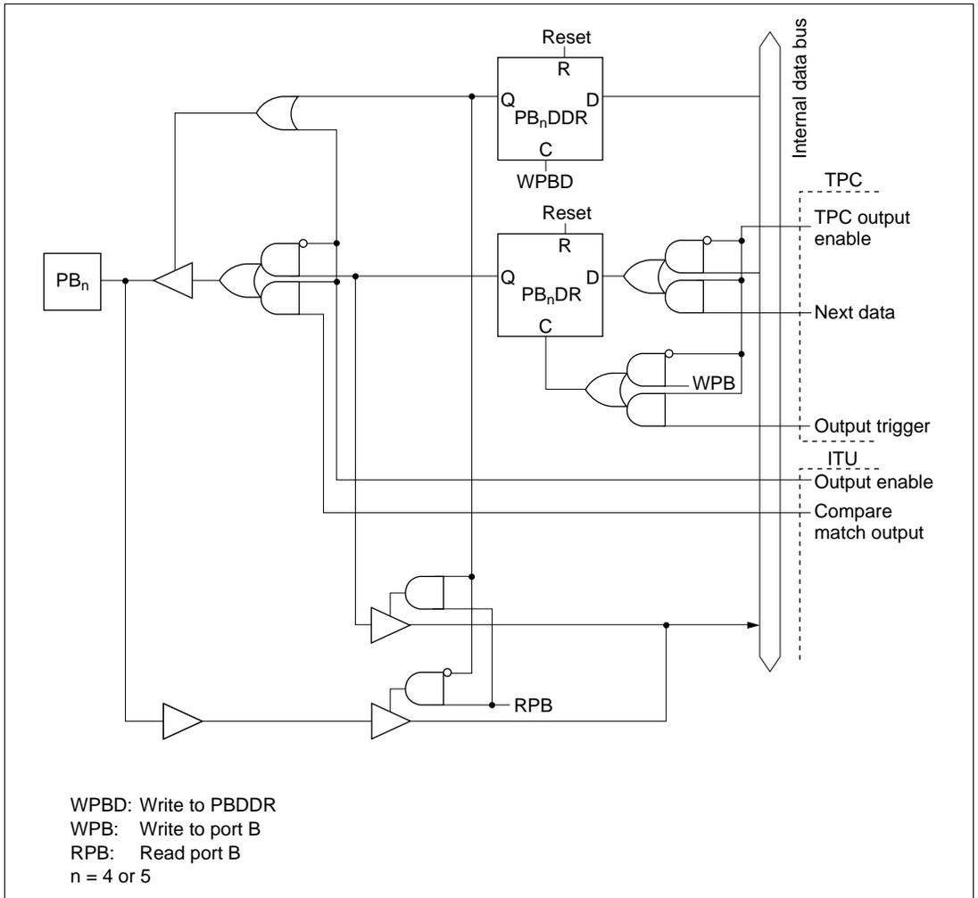
**Figure C-10 (b) Port B Block Diagram (Pins PB<sub>4</sub>, PB<sub>5</sub>)**
