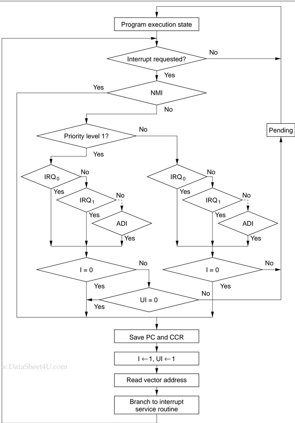
**Figure 5-6 Process Up to Interrupt Acceptance when UE = 0**
