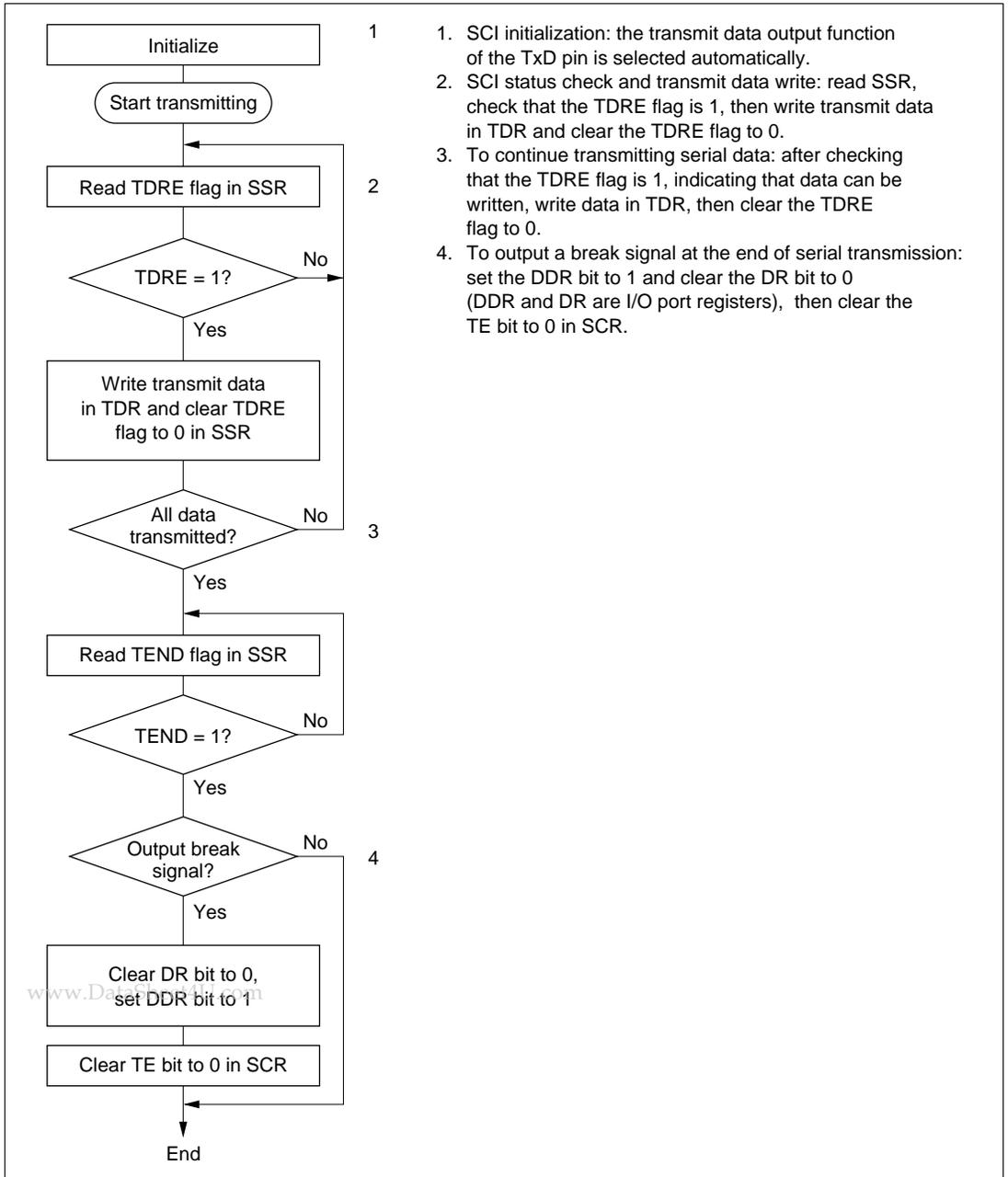
**Figure 11-5 Sample Flowchart for Transmitting Serial Data**
