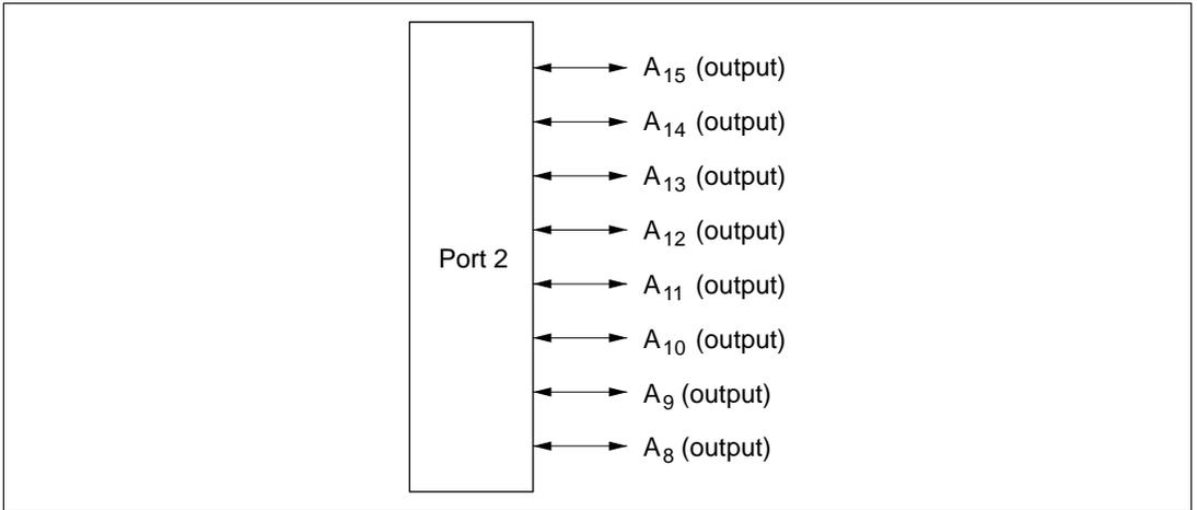
**Figure 7-6 Pin Functions in Modes 1 and 3 (Port 2)**
