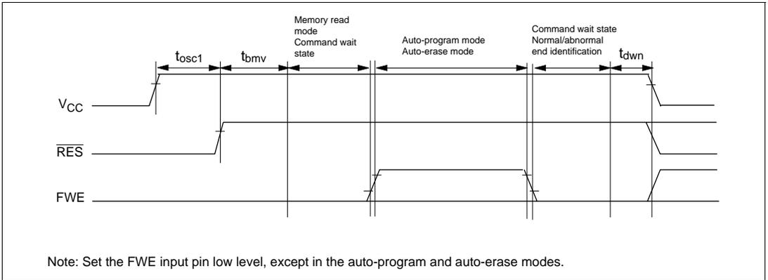
**Figure 15-23 Oscillation Stabilization Time, Boot Program Transfer Time**
