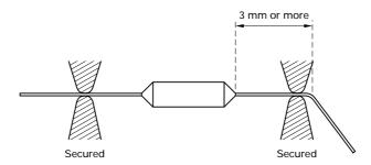
The lead wire should be bent at a distance 3 mm or more from the body of the fuse, and should not be twisted.
