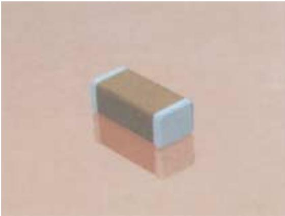
High value, low leakage and small size are difficult parameters to obtain in capacitors for high voltage systems. AVX special high voltage MLC chips capacitors meet these performance characteristics and are designed for applications such as snubbers in high frequency power converters, resonators in SMPS, and high voltage coupling/DC blocking. These high voltage chip designs exhibit low ESRs at high frequencies.
