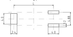
Do not design any conductive path between the pattern
