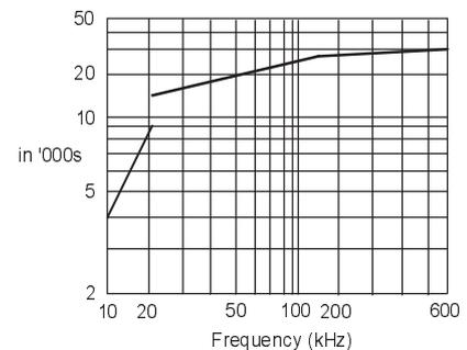
Figure 4 - CX-1H Typical Turning Point Temp. (°C)
