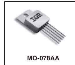
The IRUH50PA23B20 is a space qualified, ultra low dropout linear regulator designed specifically for space applications. This product has been characterized to a total ionizing dose of 200Krad(Si) per MIL-STD-883, Method 1019 at both high and low dose rates under biased and unbiased conditions to account for ELDRS effects in bipolar devices. The ultra low dropout voltage of 0.4V @ 3A makes the part particularly useful for applications requiring low noise and higher efficiency.
