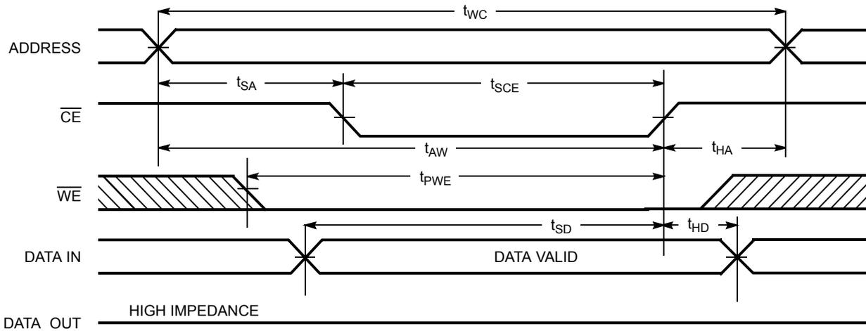
**Write Cycle No. 2 ( $\overline{WE}$  Controlled)** [16]
