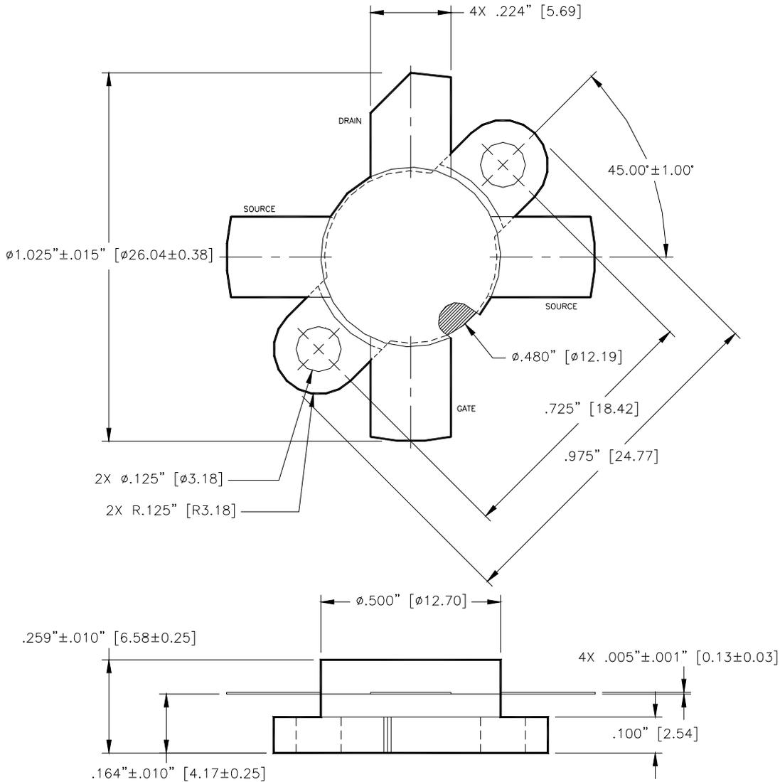
Unless otherwise noted, tolerances are inches  $\pm .005$  [millimeters  $\pm 0.13$ mm]
