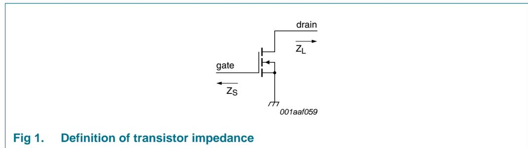
**Fig 1. Definition of transistor impedance**
