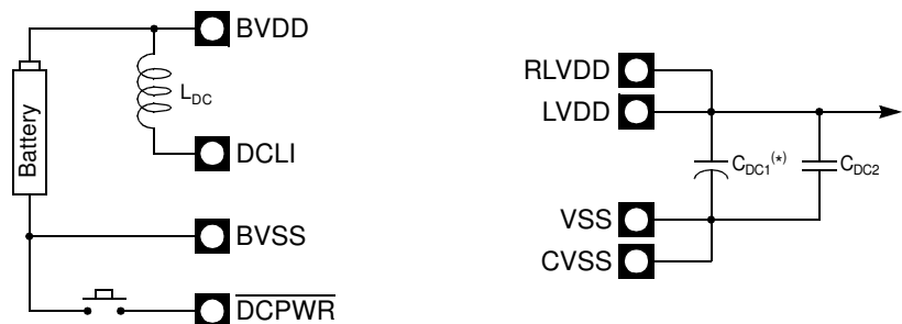
Figure 8. Battery DC-DC Connection
