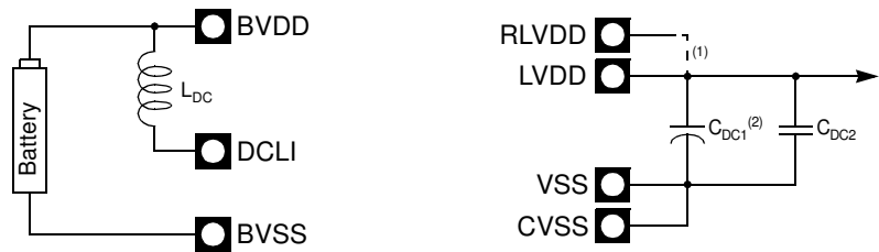
Figure 135. Battery DC-DC Connection
