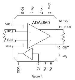
The device also includes a unity gain buffer, for the buffering of DC signals such as the common-mode-input to the amplifier. This buffer is found between pins 6 (input) and pin5 (output). If this buffer is not used, the output can be left disconnected and the input can be grounded.
