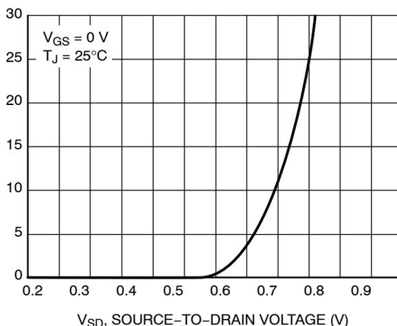
**Figure 10. Diode Forward Voltage vs. Current**
