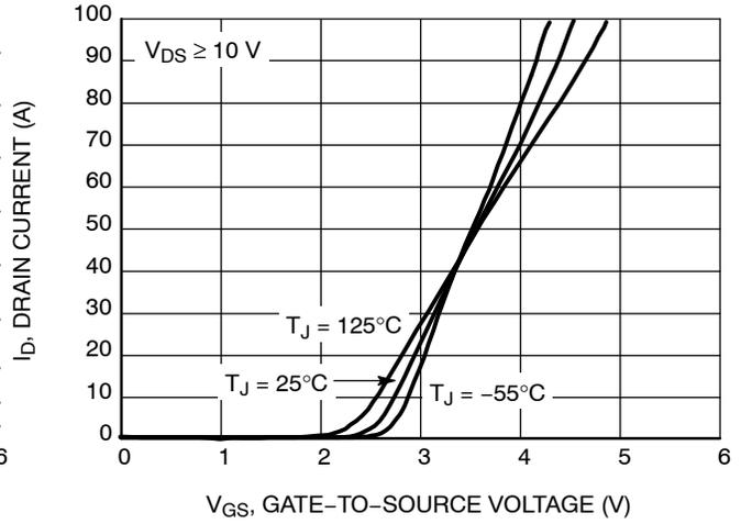
Figure 2. Transfer Characteristics
