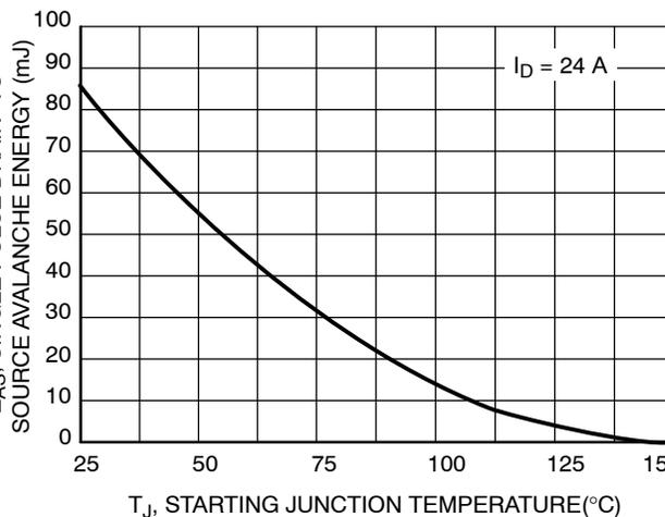
**Figure 12. Maximum Avalanche Energy vs. Starting Junction Temperature**
