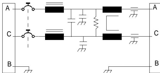
The ZG-1435-5B filter has been designed for systems operating under the requirements of MIL-STD-461C. If MIL-STD-461D or E are specified then part number ZG-1435-5BD should be specified. The difference is that the differential capacitor is repositioned on the line side in order to match the test configuration of 461D and E.
