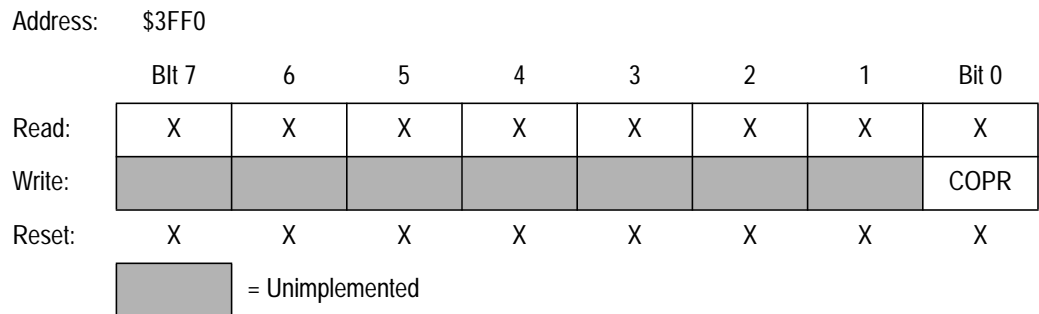
Figure 5-3. COP Watchdog Timer Location
