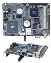
The HS-2606 is a 100/133MHz FSB VIA CLE266/VT8235 chipset-based board designed for Mini PCI Local Bus ULV Intel® Celeron® processor 400/650MHz. These features combine and make the HS-2606 and ideal all-in-one industrial single board computer. Additional features include and enhanced I/O with CF, PCMCIA, CRT/Panel, audio, LAN TV-Out, 4 COM, and USB2.0 interfaces.
