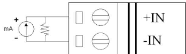
**Note:** When connecting to a current source, an optional external 125-Ohm resistor is required.
