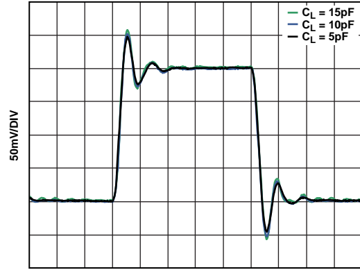
Figure 36. Small Signal Transient Response vs. Capacitive Load ( C_L ), G = 12.04 dB
