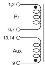
The windings are connected internally as shown
