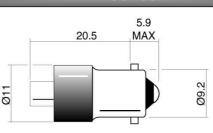
Dimensions in mm (Typical) Scale 2 : 1 Green dot on base of product indicates centre contact cathode -ve. Colour dot on sleeve denotes LED colour.
