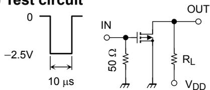
$V_{DD} = -3 \text{ V}$
