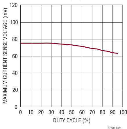
Maximum Current Sense Threshold vs Duty Cycle
