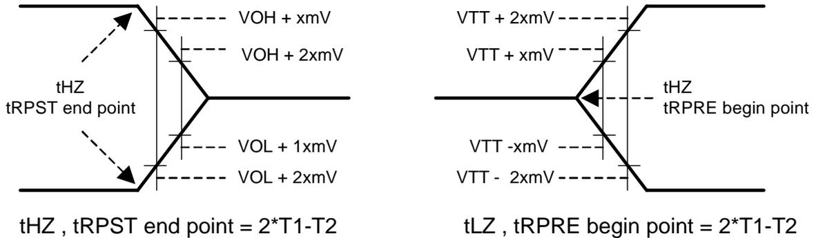
20. Input waveform timing with differential data strobe enabled MR[bit10]=0, is referenced from the input signal crossing at the  $V_{IH}(ac)$  level to the differential data strobe crosspoint for a rising signal, and from the input signal crossing at the  $V_{IL}(ac)$  level to the differential data strobe crosspoint for a falling signal applied to the device under test.
