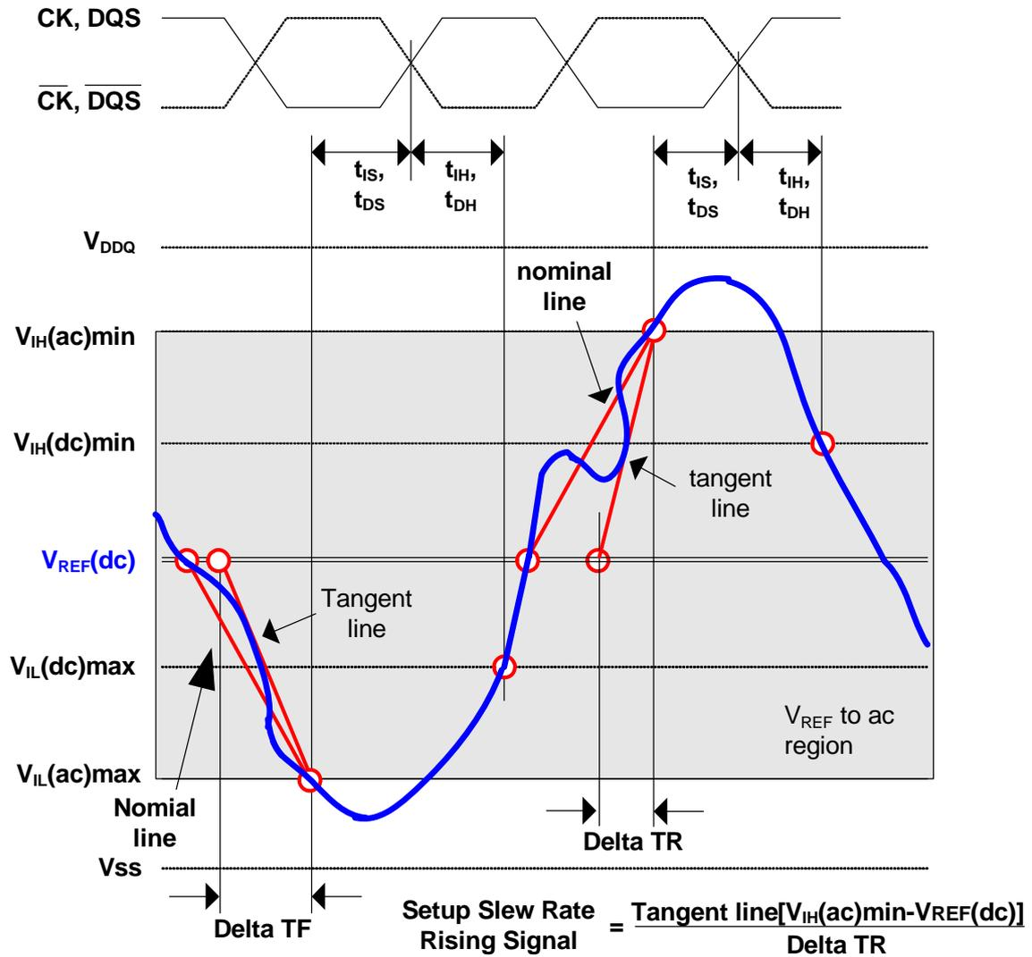
$$\text{Setup Slew Rate Falling Signal} = \frac{\text{Tangent line}[V_{REF(dc)}-V_{IL(ac)max}]}{\text{Delta TF}}$$
