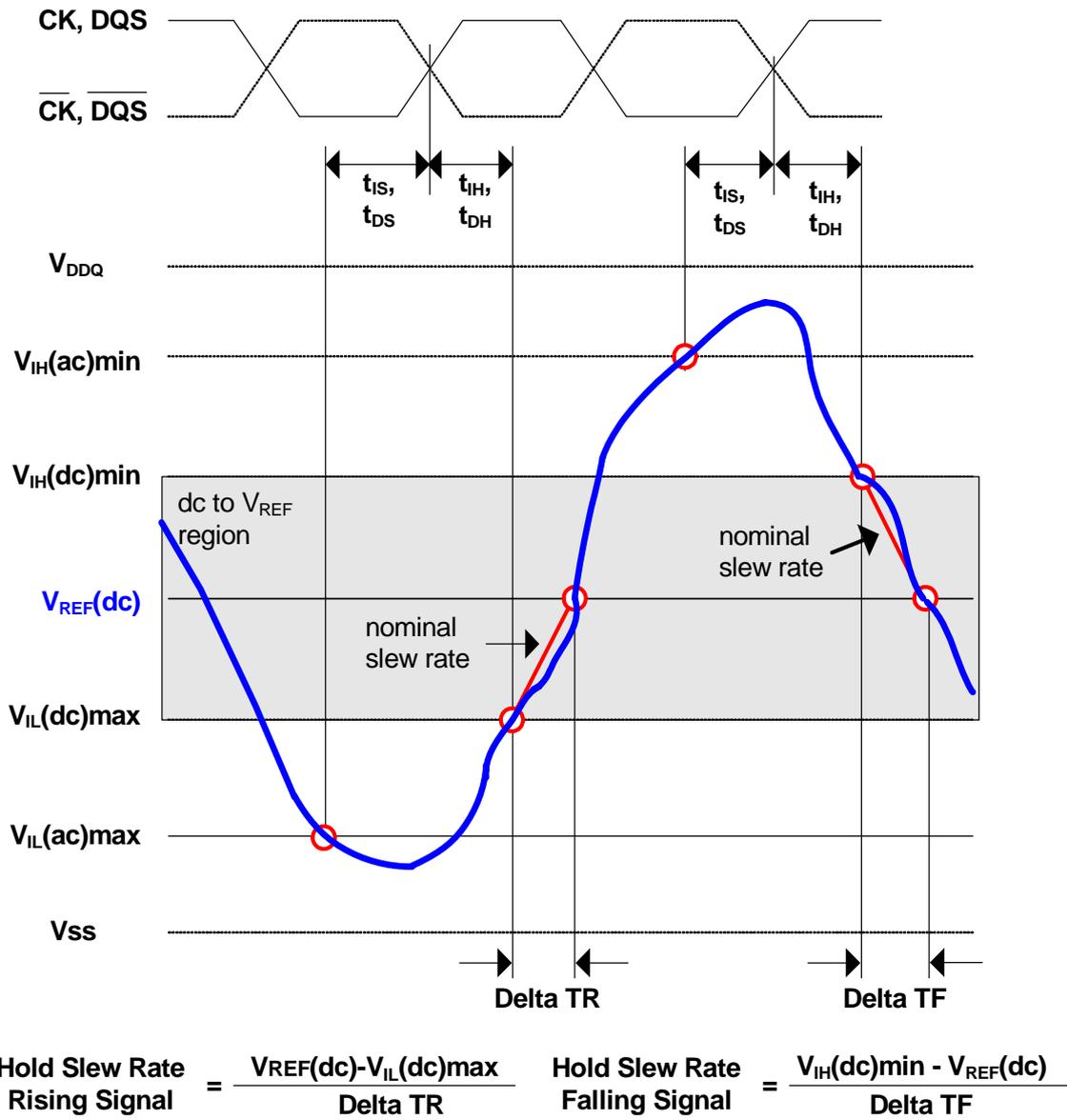
Fig. -d Illustration of tangent line for tIH , tDH
