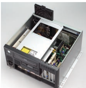
Solid disk drive housing & easy-to-maintain fan filter
