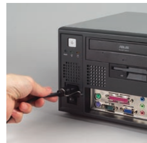
Plug ring-lock securely fastens the power cord
