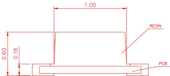
For reflow soldering
