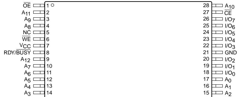
TSOP Package (8mm x 13.4mm) (H13)
